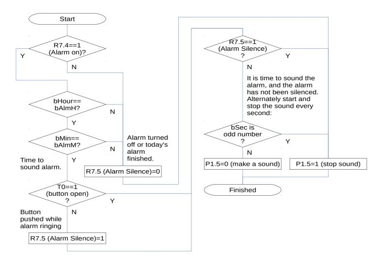
Flag R7.4 will be used as the "Alarm On" flag. When it is logic 1, the alarm is on.
