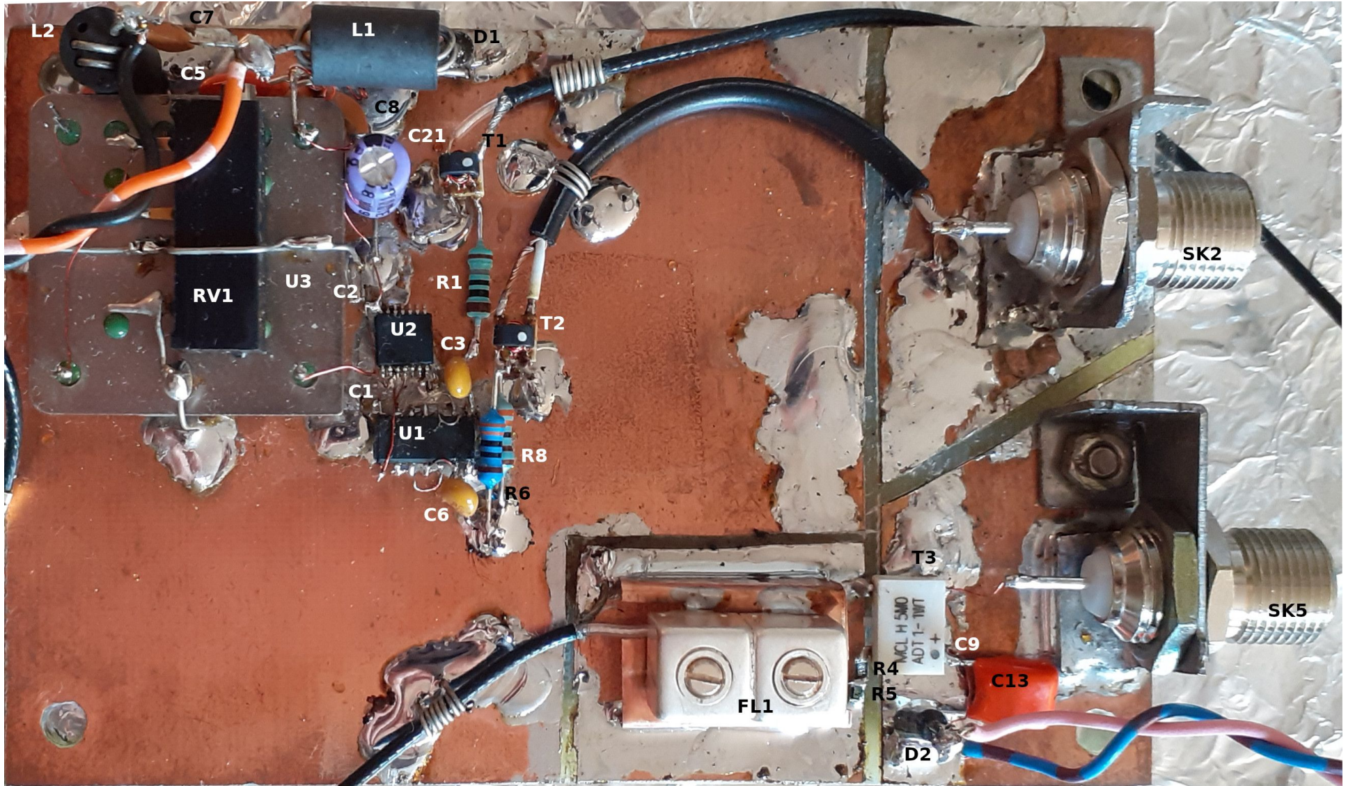
Figure 13: Layout of the frequency reference PCB.
