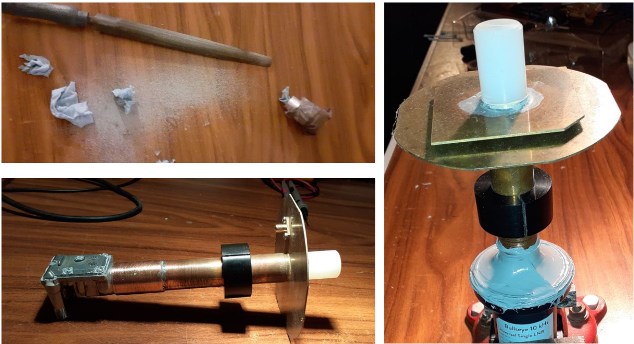
Figure 60: Fitting the LNB into the 22mm POTY pipe joint.
