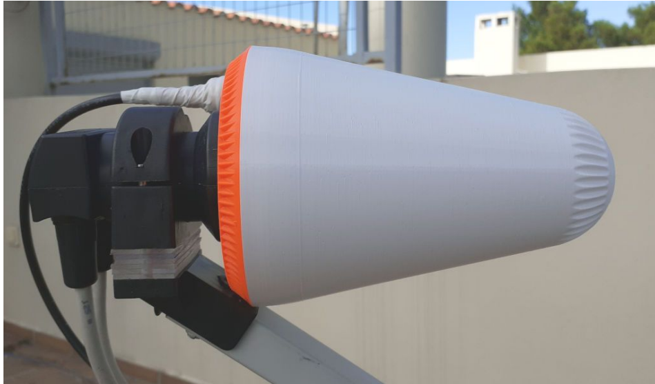
Figure 27: LNB end of the satellite dish arm, showing how the LNB support has been lifted with a stack of six sheets of perspex, increasing the clearance to allow for installation of the Ice Cone v2.1.
