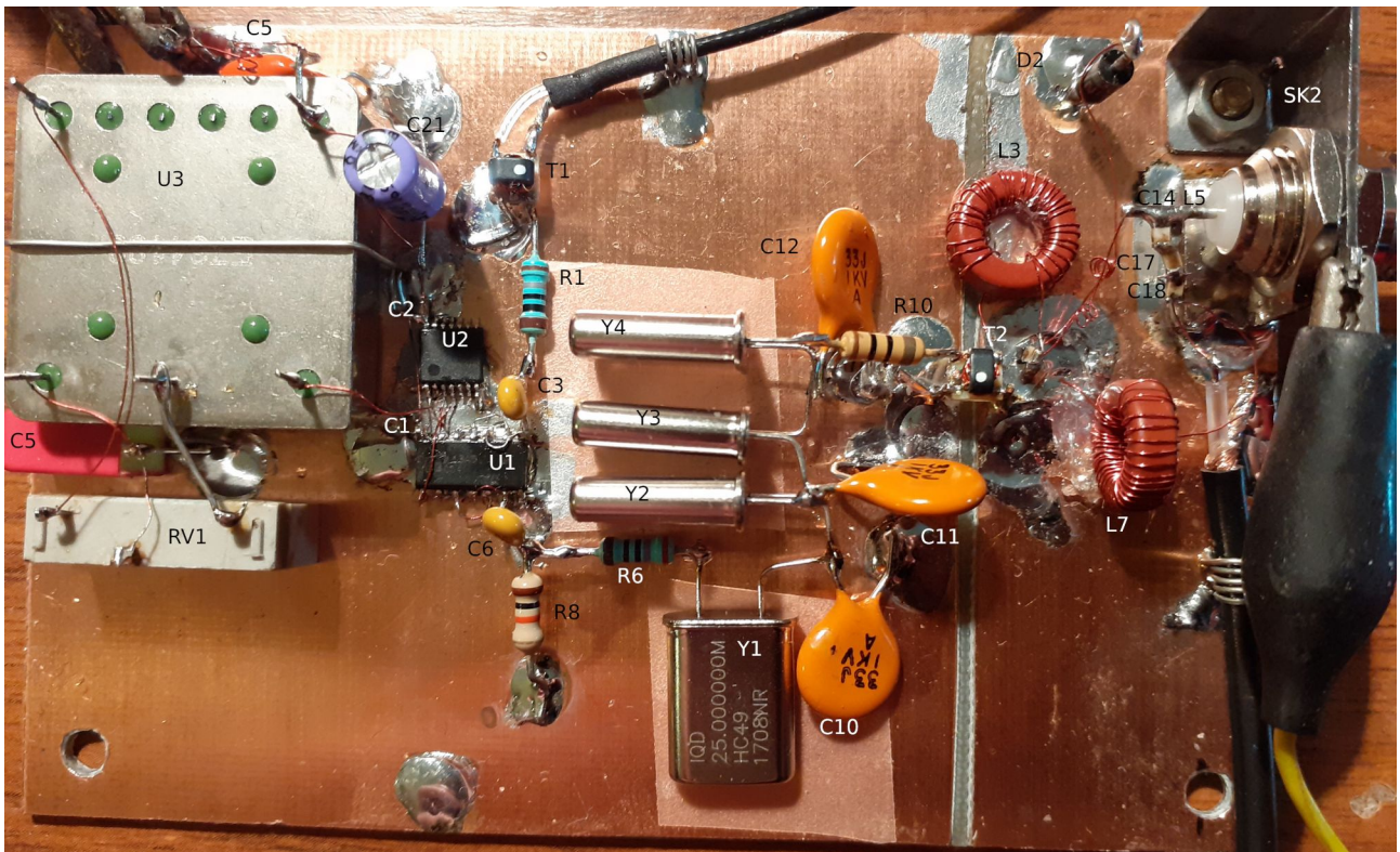
Figure 56: Layout of the frequency reference PCB for the for the Amiko L107 single-receptacle LNB. Note that this is a somewhat earlier incarnation which does not include C7, C13, L1.
