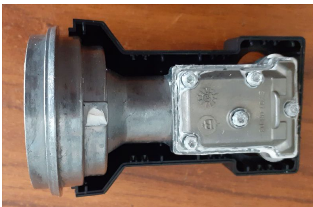
Figure 25: Othernet Bullseye with front cover removed (top left) and shell removed.
