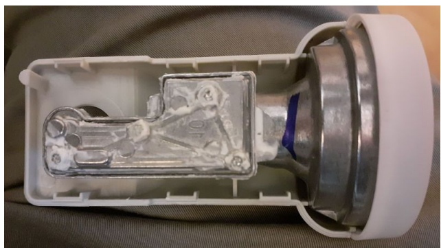
Figure 53: Amiko L107 with the plastic cover removed.
