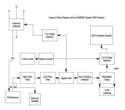
shown in figure 1. - Zero crossings of the Doppler frequency shift pattern correspond to the antenna position located directly toward the source of transmission (position A) or directly opposite the source of transmission (position C). The zero-crossing signal passes through an adjustable delay before it latches the direction indicating LED. The adjustable delay is used to calibrate the LED direction indicator with the actual direction of the transmission.
