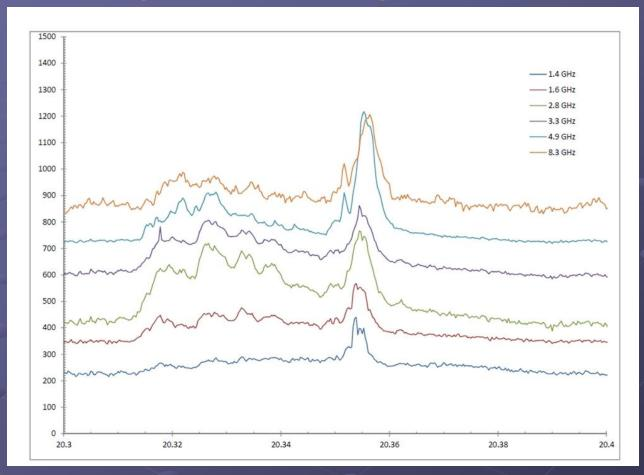
Measurement from new Solar Flux instrument at DRAO in Penticton BC. The big spike is a M-Class solar flare. The increase in noise before the flare is also caused by the sun. At no point do we see the moon shadow effect we expected to see.
