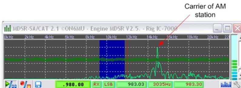
After tuning in a local AM station the SA (spectrum analyzer) will display the following spectrum as seen above. The audio in the speaker will be crackling or there will just be noise.
