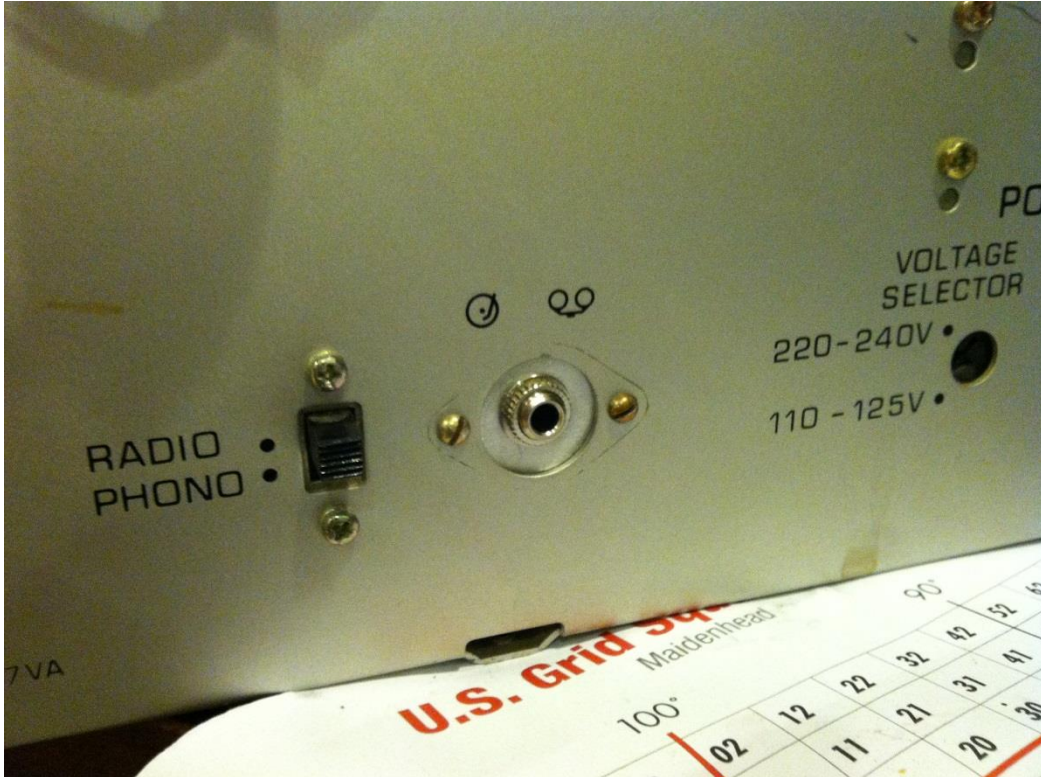
Figure 4 – Output port, modified for 3.5mm mono audio jack.
