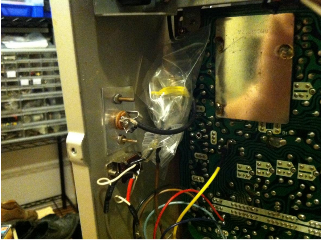
Figure 5 Inside-case view of 3.5mm jack. Stock components bagged and taped radio can be returned to stock configuration.
