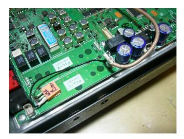
Solder the ground shield of the RG174 to the first 3 pins of J23. This will also make the option filter 1 selectable in the radio's menu. Pin 4 is the RF and it needs to be connected to the center of the RG174 coaxial cable and to the input of the 455kHz filter. The center pin of the filter is connected to pin 2 of J24 and the output is connected to pin 3. The filter is secured on the PCB with double sticky tape. The filter will keep the AGC function
