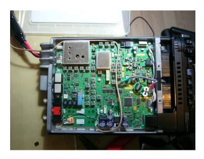
The best routing of the RG174 is shown below for the FT-897. The LIF PCB can be mounted inside the transceiver. The PCB has to be made slightly smaller to fit into the gap, as shown, with sand paper. Power is provided though the regulator IC on the upper PCB. Use the +12V side of the regulator IC. The LIF PCB has its own regulator.
