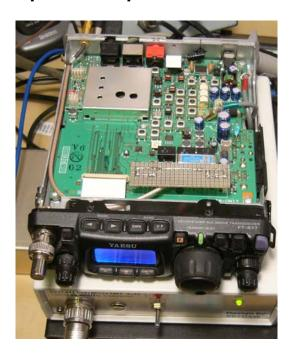
A small circuit board serves as a platform to solder the 0.075" spacing strip connector as well as a 47pF capacitor.
