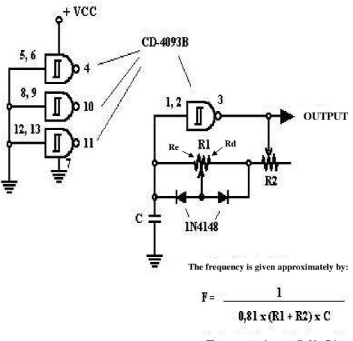
The symmetry is controlled by R1 The frequency is controlled by R2
