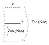
The manufacturer specifies the output impedance between terminals 'a' and 'b' and between terminals 'a' and 'c'. We want to know the output impedance between terminals 'b' and 'c'.
