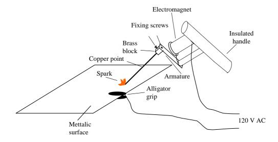
The brass block, fixed to the end of the armature with a screw, can be got from an old AC wall switch or inlet, as they just use brass blocks for connection to the wires.
