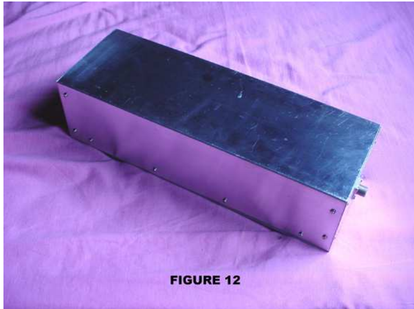
In Figure 11 is the bottom view of the box already closed, where we can see the plastic feet. Figure 12 shows the filter box view in normal position. Its dimensions are 45cm x 15cm x 12cm and aluminum made.
