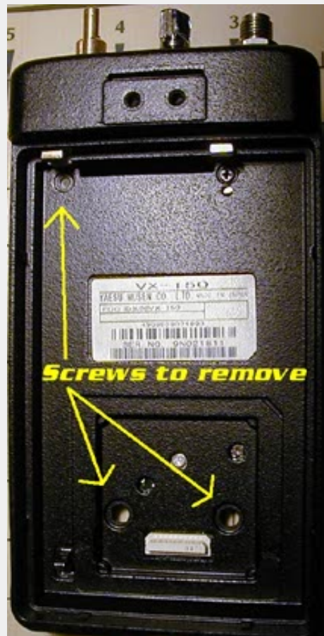
Fig 2 Remove screws
