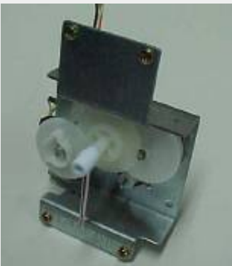
Photo 3: Mechanical indicator needle system
