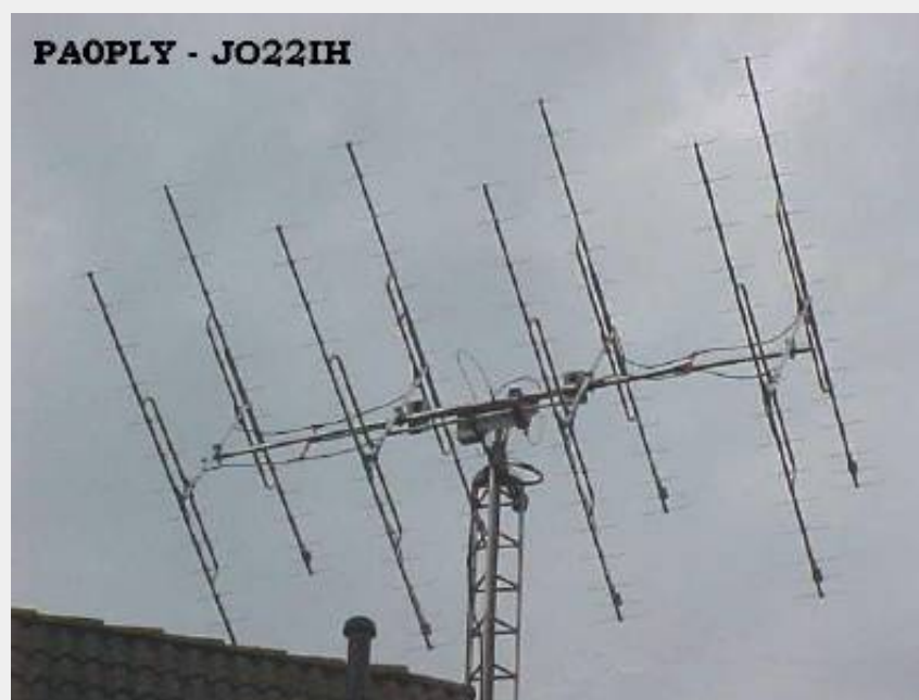
Photo 1.: Large EME array for 432MHz.
