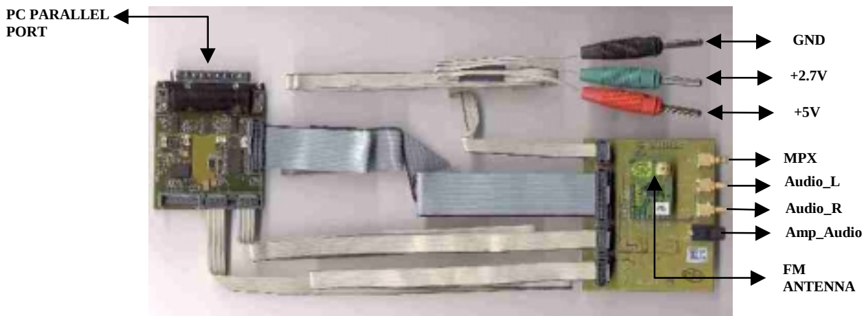
Figure 34 connection of TEA5767/68 demo board
