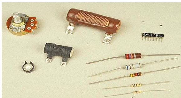
Figure 20 - Different types and values of resistors. Photo by KF5WT
