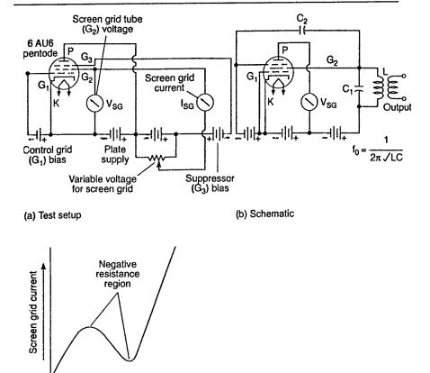
Fig. 2.16 Negative resistance in the transitron circuit
