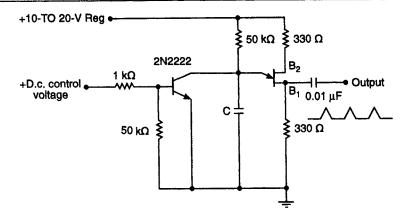
Simple voltage-controlled oscillator using a unijunction transistor. The bipolar transistor is used as a variable resistance to delay the charging rate of timing-capacitor C
