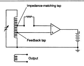
Basic Lampkin oscillator. One objective sought is to attain an approximate impedance match between the input of the amplifier and the resonant tank
