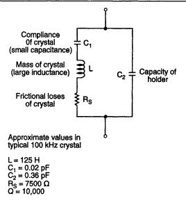
Fig. 1.27 Equivalent circuit of a quartz crystal
