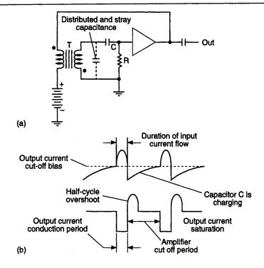
Basic operation of the blocking oscillator. a, Circuit. b, Fia. 3.17 Waveforms
