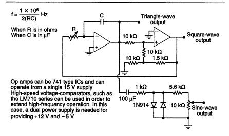
**Fig. 5.16** A basic function generator using general-purpose op amps. This type of oscillator provides optional outputs of square, triangular or sine waves
