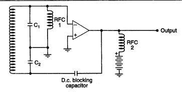
The shunt-fed Colpitts oscillator. The capacitive divider formed by  $C_1$  and  $C_2$  is the hallmark of the Colpitts circuit. The quality of the radio frequency chokes is important in the shunt-fed version. RFC1 is usually optional; if used, the two chokes should be different types to avoid an undesired resonance
