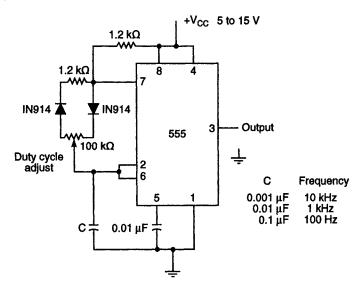
The 555 timer IC connected to provide adjustable duty cycle at fixed frequency. The arrangement is such that the sum of charge and discharge times of capacitor C remains constant as each is varied by the potentiometer. The adjustable range of the duty cycle is approximately 1-99%
