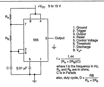
Circuit of the astable or multivibrator mode for the 555 IC timer. Fig. 6.18 Minor modifications of this basic oscillator leads to various useful applications. By impressing different modulating voltages at terminal 5, the output waveform and frequency can be controlled to produce such functions as frequency divider, pulse-width modulator, pulse-position modulator and emulation of sounds, such as that of a siren
