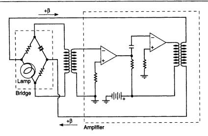
**Fig. 4.16** The Meacham bridge oscillator. Operating very close to balance, the bridge automatically regulates feedback, thereby maintaining Class-A amplifier operation, exceptional frequency stability and good wave purity
