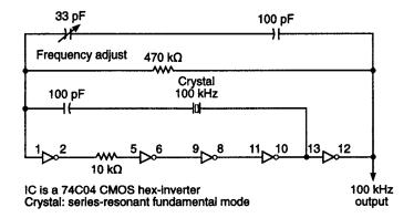
**Fig. 5.22** 100 kHz oscillator using five sections of a CMOS hex inverter. Circuits of this kind employing several cascaded stages develop high feedback and can sometimes generate self-excited oscillations if the crystal is defective or is not in place
