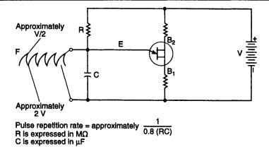
Fig. 2.18 Basic unijunction relaxation oscillator
