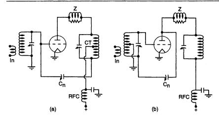
Simplified neutralizing circuits in electron-tube radio frequency amplifiers. Both techniques apply phase-reversed voltage to the internal feedback-path, thereby cancelling the positive-feedback from the plategrid capacitance. Cn is the neutralizing capacitor, set to approximate plateto-grid capacitance. a, Plate neutralization circuit. b, Grid neutralization circuit
