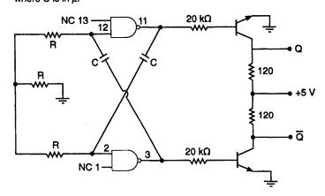
ICs are two sections of quad-NAND gate SN7400 Transistors are 2N2222 or similar 'workhorses' Pin 7 on the SN7400 connects to ground and pin 14 connects to +5 V
