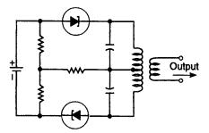
Fig. 3.5 Cascade tunnel-diode oscillator
