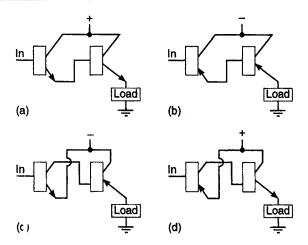
The four Darlington circuits using bipolar transistors. The output device may or may not be a power transistor. Because of the high input impedance and high current gain of these pairs, they are particularly suitable for RC oscillators such as the phase shift, the parallel T and the Wien. (a) npn pair, (b) pnp pair, (c) npn input, pnp output, (d) pnp input, npn output.
