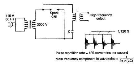
Fig. 2.14 A spark-gap oscillator
