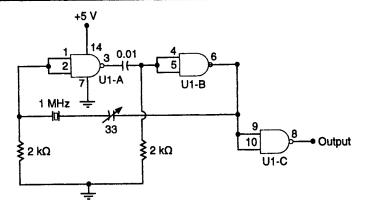
U1-A, U1-B and U1-C are three sections of an SN7400 quad NAND gate
