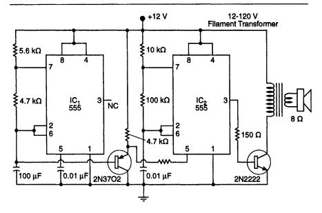
Dual oscillators arranged to operate as an electronic siren. The low-frequency ramp from IC<sub>1</sub> modulates the higher frequency (500 Hz) oscillator, IC2. The oscillation frequency of IC2 is caused to vary above and below its natural 500 Hz frequency, thus emulating the familiar wail of the police siren
