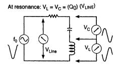
Fig. 1.18 Voltage step-up in a resonant series tank circuit
