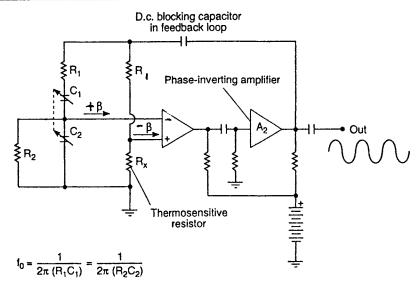
Fig. 3.21 Basic Wien bridge oscillator. When properly designed, excellent sine waves are produced by this circuit
