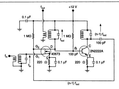
Basic circuit of a regenerative modulator. A wide spectrum of audio and radio frequencies can be readily accommodated. LC resonances and parameter values are not critical. If sufficient drive-level exists, the operation is reliable and jitter-free. Unlike flip-flop frequency dividers, this circuit delivers a sinusoidal output
