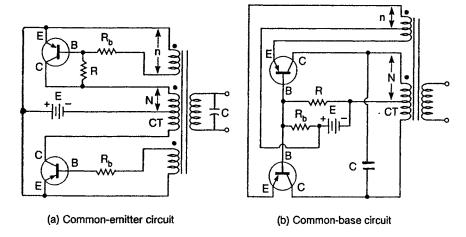
Fig. 2.22 Saturable-core oscillator circuits
