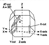
Fig. 1.30 Temperature coefficient and other characteristics depend upon the angle of cut. The AT-cut is processed approximately at 35° with respect to the Z-axis. Minor angular deviations of this cut enables 'fine-tuning' of the temperature coefficient. The X-cut is made perpendicular to the X-axis. The Y-cut is made perpendicular to the Y-axis. Many other cuts have been used, each with its unique parameters and performance trade-offs
