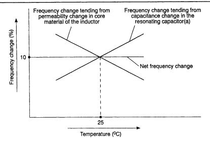
Idealized temperature compensation of frequency change. Core materials such as the much-used No. 6 and 7 iron-powder toroids exhibit a temperature coefficient. The frequency decrease temperature that tends from this characteristic can be counteracted by appropriate choice of capacitors with a negative temperature coefficient. Precisely-characterized ceramic capacitors are often used, but sometimes polystyrene capacitors prove suitable
