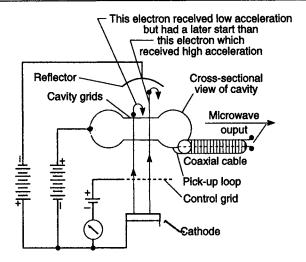
Basis for oscillation in the reflex klystron Fig. 2.24
