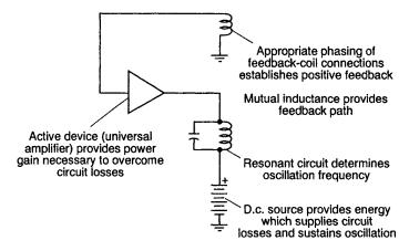
Fig. 3.8 Function of the elements in a feedback oscillator
