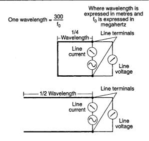
Simplest resonant lines for simulating the properties of the parallel-tuned tank circuit
