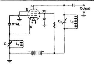
Fig. 4.14 The tri-tet oscillator
