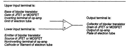
Fig. 2.27 The universal amplifier symbol. Inasmuch as most oscillators can be made to operate with a variety of active devices, it is too restrictive to discuss the operating principles in terms of a single device. The triangle symbol is commonly used to depict all kinds of amplifiers and is, therefore, appropriate for use with oscillator circuits
