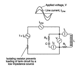
Fig. 1.12 Resonance conditions in a typical LC tank circuit
