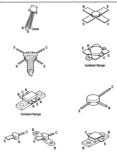
**Fig. 6.23** Unique package styles for UHF and microwave transistors. The primary purposes are to ensure stability in amplifier circuits. However, the packaging has considerable influence on the efficiency of oscillators. Multiple E and B connections reduces lead resistance and inductance. Specific geometric arrangements favour optimum performance in common emitter, common base or common collector circuits
