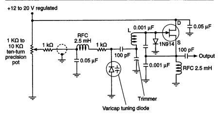
Fig. 5.11 Example of varicap tuning of an oscillator. This arrangement shows the general features of varicap tuning for the amateur HF bands. Various varicaps are available for optimum results, but ordinary signal diodes often work well
