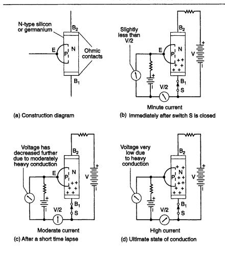
Fig. 2.17 Conduction states in a unijunction transistor
