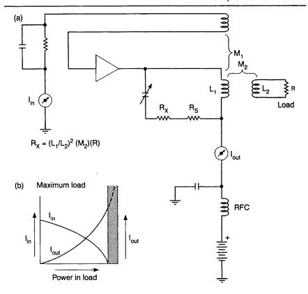
**Fig. 3.23** Loading characteristics of an LC feedback oscillator. a, Circuit:  $R_x$  is load reflected into LC tank. b, D.C. currents in oscillator. Oscillator no longer is operative in shaded region because of overloading and load power falls to zero
