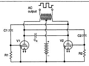
Fig. 2.12 Basic thyratron inverter
