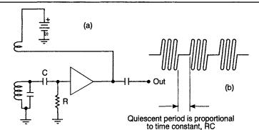
Fig. 3.18 The squegging oscillator. a, Circuit. b, Waveform
