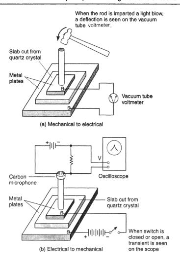
Fig. 1.26 Experiments for demonstrating the piezoelectric effect
