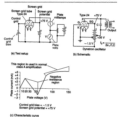
Fig. 2.15 Negative resistance in the dynatron circuit
