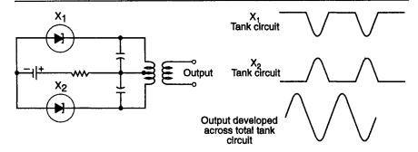
Fig. 3.4 Push-pull tunnel-diode oscillator and waveforms
