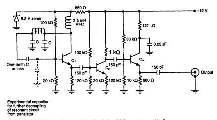
Q<sub>1</sub>, Q<sub>2</sub> and Q<sub>3</sub> are 2N2222 or similar transistors. An MPF102 JFET can also be used for Q<sub>1</sub>
