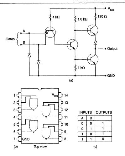
Circuit, pin-out and truth table of the SN7400 NAND gate. This Fig. 5.18 device is typical of logic ICs used in oscillators, a, Internal circuit of the SN7400. Note dual-emitter input transistor. b, Pin-out of the SN7400. Note common power supply provision. c, Truth table
