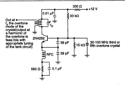
Overtone oscillator with provision to discourage fundamental frequency oscillation. The inductance of RFC must be large enough to permit operation at fo, the overtone mode, but small enough to prevent oscillation at the fundamental frequency of the overtone crystal
