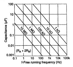
Fig. 6.19 RC combinations for attaining various frequency-ranges in the 555 multivibrator. It is a good idea to select RC combinations which avoid the use of either extremely high or extremely low values of the resistance or capacitance. Also, if an electrolytic capacitor is used, it should be a high-quality, low-leakage type. Solid-state tantalum types are especially suitable
