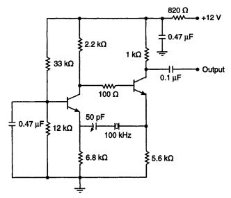
Suitable transistors include, 2N2222, 2N697, 2N708, HEP50
