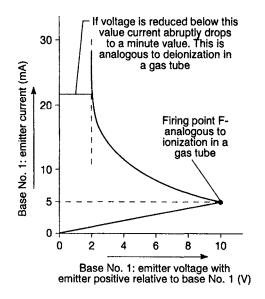
Fig. 2.19 Current-voltage relation in Base No. 1-to-emitter diode
