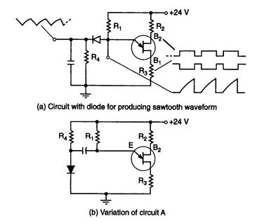
Fig. 4.24 Unijunction transistor multivibrator circuits
