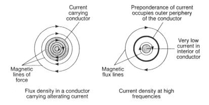
Flux-density from A.C. in a conductor and the high frequency skin-effect. At low frequencies most of the current flows throughout the cross-section of the conductor. At high frequencies, almost all current is in the outer 'skin' of the conductor
