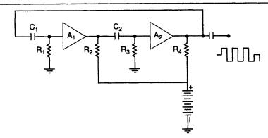
The multivibrator relaxation oscillator. The pulse repetition rate Fig. 3.16a is approximately  $\frac{1}{R_1C_1 + R_3C_2}$  Hz.
