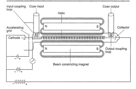
Fig. 2.25 Travelling-wave tube
