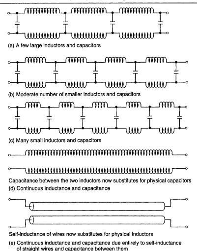
Fig. 1.23 Synthesis of a resonant transmission line from lumped elements
