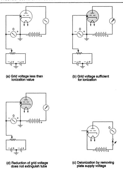
Fig. 2.11 Control of gas tubes
