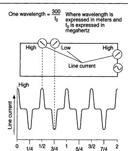
Fig. 1.19 Parallel- and series-type resonances in a short-circuited line
