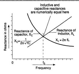
Fig. 1.9 Variation of inductive and capacitive reactance with frequency
