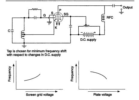
**Fig. 3.24** Basic electron-coupled oscillator and curves showing frequency variation
