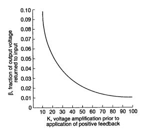
Fig. 3.10 Minimum feedback signal required for oscillation
