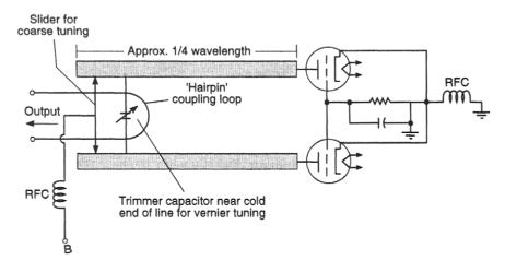
Fig. 4.17 A line oscillator for UHF
