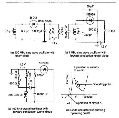
Fig. 3.6 Tunnel-diode oscillators
