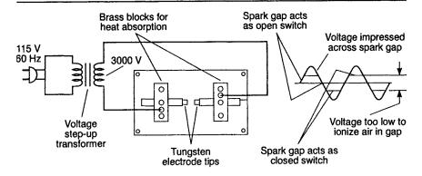
Fig. 2.13 The spark gap as a switching device
