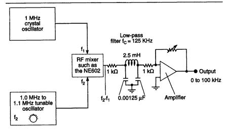
**Fig. 6.22** Basic set-up for a wide-range signal generator. Two oscillators are used. One is fixed frequency, the other is variable frequency. The generated signal is the difference frequency produced by the nonlinear mixing of the two oscillator frequencies. In principle, the output range can extend from zero frequency (d.c.). In practice, 100 Hz or so is readily obtained. Lower frequencies require special attention to the mixer and to the amplifier
