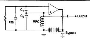
Colpitts oscillator with crystal substituted for parallel-tuned tank Fig. 4.9
