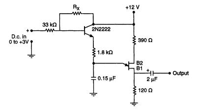
Fig. 5.26 Another unijunction VCO circuit. In this arrangement, the bipolar transistor acts as a voltage-controlled resistance in the series-charging path of the timing capacitor. Experiment with  $R_{\star}$  for best results; 330  $k\Omega$  is a good starting value
