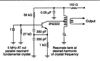
Example of harmonic oscillator. In the above circuit, all frequency Fig. 5.7 multiplication takes place within the transistor and is governed by the resonance of the output tank circuit. The position of the collector tap should be empirically optimized for highest output of the desired harmonic frequency
