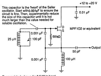
Resonant tank shown for 3.6 MHz band
