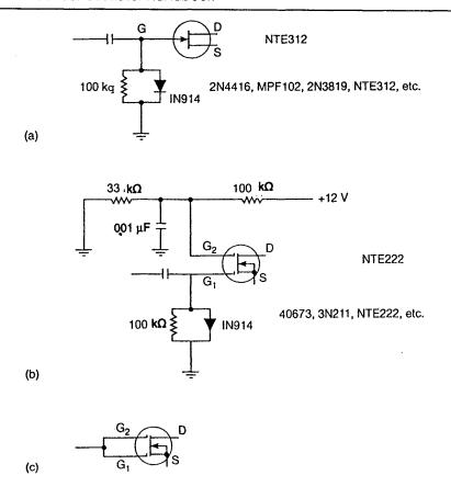
**Fig. 6.2** Methods of implementing field-effect devices in oscillators. a, JFET gate connections. The main purpose of the diode is to prevent forward conduction in gate of the JFET. b, Dual-gate MOSFET connection. The main purpose of the diode here is to limit oscillation amplitude in order to improve waveform and frequency stability. c, Alternative way to use the dual-gate MOSFET. This often amounts to a direct replacement of a JFET.
