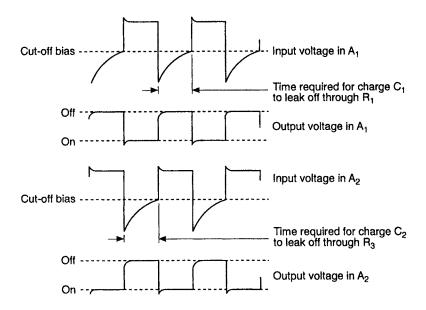
Fig. 3.16b Waveforms in multivibrator oscillator
