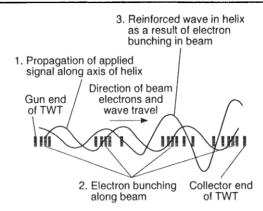
Fig. 2.26 Wave generation in a travelling-wave tube
