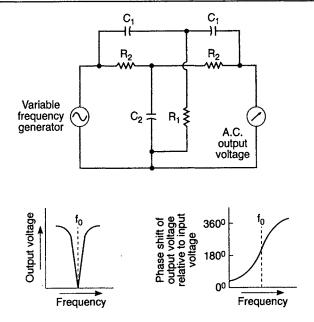
Fig. 1.38 The parallel-T network
