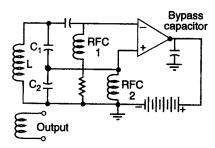
The Colpitts oscillator (series feed). Here again, RFC₁ is usually optional. If used, the two chokes should be different types
