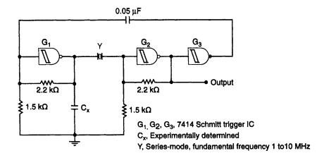
**Fig. 5.23** Crystal oscillator using Schmitt trigger logic elements. This is a vigorous square-wave oscillator. The function of  $C_{\mathsf{x}}$  is to discourage generation of spurious frequencies
