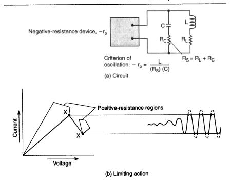
Limiting in a negative-resistance oscillator Fig. 3.15
