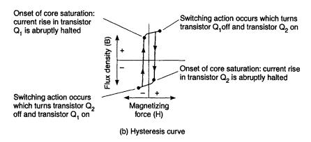
Fig. 2.21 The saturable core as an oscillation-provoking device
