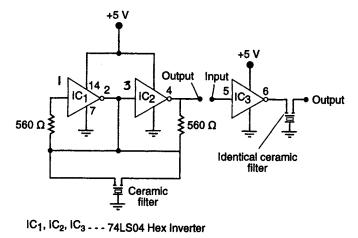
Fig. 6.6 A ceramic-filter oscillator circuit. Shown also is an optional stage
