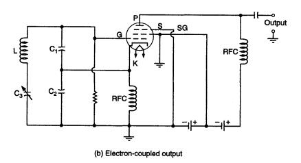
Fig. 4.13 Clapp oscillators
