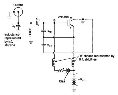
Equivalent circuit of the stripline microwave oscillator of Fig. Fia. 6.25 6.24. This is a Clap, series-tuned oscillator of the Colpitts family. Parallel resonance mode operation is also possible, but impedance considerations favour the series mode. Adjustments of  $C_1$  and  $C_2$  are made not only to generate the desired frequency, but to also approach an output impedance of  $50\Omega$
