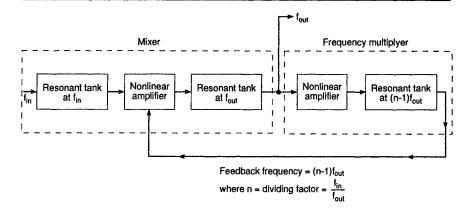
**Fig. 6.7** Block diagram of the regenerative modulator. Although an internal frequency-multiplication is performed, the overall operation is frequency division. Like a true oscillator, such an arrangement requires energy feedback for its operation
