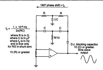
The parallel-Toscillator. Also known as the twin-Toscillator, this circuit is much used in low and audiofrequency applications. It is capable of exceptionally good wave purity. Note that oscillation occurs at a higher frequency than fo
