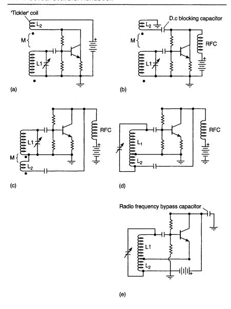
**Fig. 4.1** Evolution of Type-1 Hartley oscillators from basic tickler feedback circuit. a, Tuned base tickler oscillator. b, Tuned base tickler oscillator with shunt d.c. feed. c, Circuit b with physical rearrangement of tickler coil. d, Shunt-fed Hartley (hot collector) oscillator. e, Series-fed Hartley (hot emitter) oscillator
