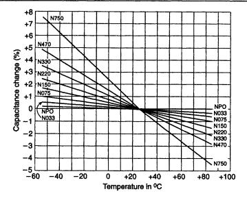
**Fig. 6.4** Standard selection of negative temperature-coefficient ceramic capacitors. Capacitors with appropriate capacitance and temperature coefficients can go a long way in reducing temperature-dependent frequency drift in oscillators. Note that the temperature coefficient of the NPO capacitor is zero. Experimentation often involves combining the NPO capacitor with one of the other. One strives to optimize frequency stability, and at the same time retain desired tank-circuit tuning
