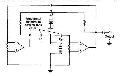
Fig. 4.20 Basic Franklin oscillator
