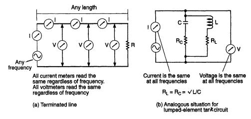
Termination of line by resistance equal to its characteristic Fig. 1.24 impedance destroys resonance completely
