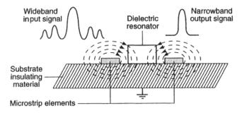
Fig. 1.33 Coupling mechanism and filtering action of a dielectric resonator. The radio frequency magnetic fields provide energy linkage into and out of the dielectric resonator, which behaves as a selective filter
