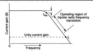
Current gain vs frequency of bipolar radio frequency transistors. The slope of the gain decline is at least 6 db per octave (20 db per decade). The excess gain at low frequencies makes transistor radio frequency amplifiers vulnerable to low-frequency parasitic oscillations
