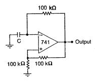
Fig. 5.13 A square-wave oscillator suitable for a wide variety of op amps. A 50% duty cycle multivibrator type square-wave generation results from alternate turn on and turn off of the op amp
