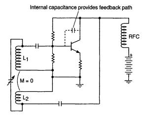
**Fig. 4.2** The Type-2 Hartley oscillator. Oscillation takes place despite the fact that there is no inductive coupling between the input and output circuits
