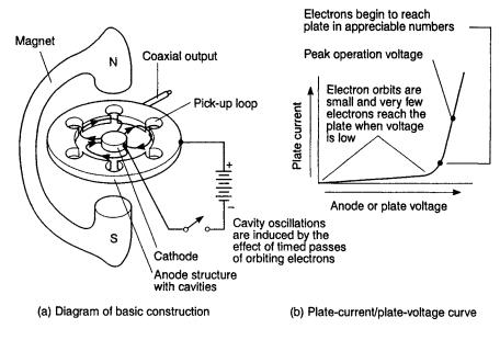
Fig. 2.23 Multicavity magnetron
