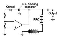
Fig. 4.11 The Pierce crystal oscillator
