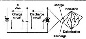
Fig. 2.9 Gas-diode relaxation oscillator
