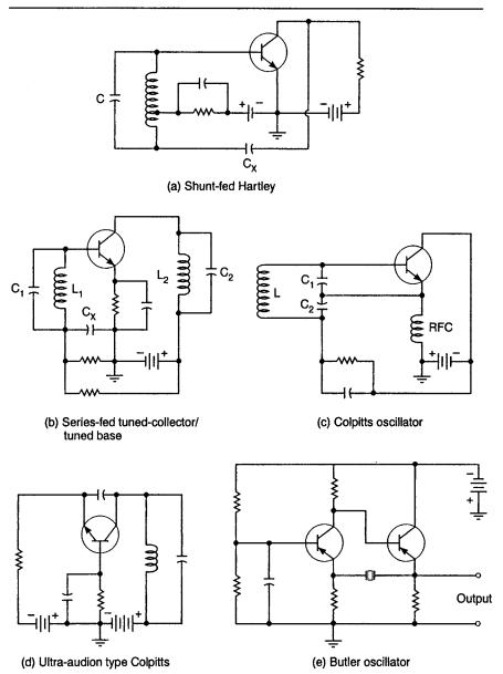
**Fig. 4.22** Representative oscillators using bipolar transistors. Usually a bit of experimentation will pay dividends in optimizing operation for stability, self-starting, wave purity, power output, etc. D is another version of the circuit of Fig. 4.10
