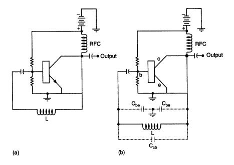
The ultra-audion oscillator: a member of the Colpitts family. a, Basic hardware circuit. b, The equivalent circuit. The configuration of the internal capacitances form a Colpitts-type oscillator
