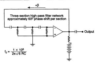
$f_0$  is in Hz when R is expressed in ohms, C is expressed in  $\mu F$
