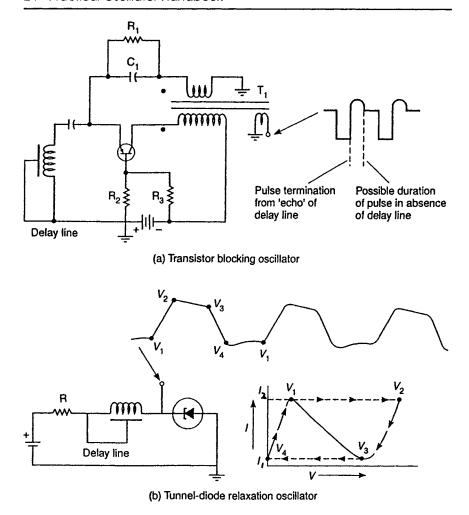
Fig. 1.22 Stabilization of wave duration by use of delay lines
