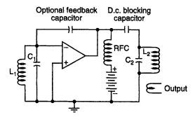
Tuned-output/tuned-input oscillator. In this shunt-fed circuit, the choke must not resonate with the LC tanks. (Because of their distributed capacitances, radio frequency chokes exhibit several series and paralleltype resonances)
