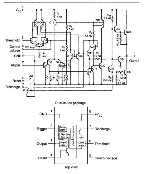
Circuit and simplified block-diagram of the 555 IC timer. Despite the high number of active-devices, the IC is easy to implement in useful oscillator-related applications
