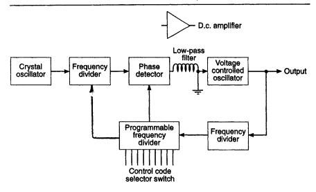
Block diagram of a practical PLL. A set-up such as this allows manual selection of many stabilized frequencies. Also, the individual functional-blocks operate within constraints favourable to optimum performance and cost considerations. The symbolically-depicted low-pass filter is often an RC type. A d.c. amplifier may follow the phase-detector
