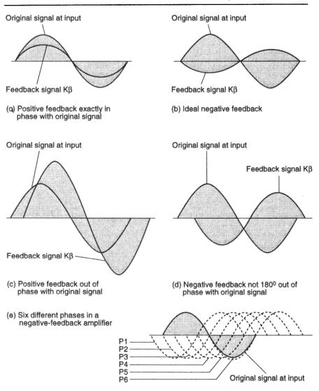
Fig. 3.12 Various feedback conditions in amplifiers and oscillators
