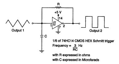
The Schmitt-trigger oscillator. The duty cycle is inherently 50%. Experiments can start with  $R = 100 k\Omega$  and  $C = 0.01 \mu F$ , corresponding to a frequency of several kHz. The exact frequency will depend upon the upper and lower trip points of the Schmitt trigger. Triangular Output 1 is vulnerable to loading and is best sampled through a buffer stage
