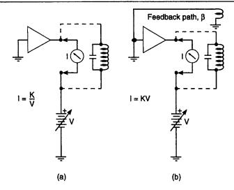
Comparison of negative-resistance oscillator and feedback oscillator. The negative-resistance device displays negative-resistance without external feedback, a, Negative-resistance oscillator, b, Feedback oscillator
