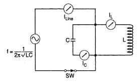
Fig. 1.8 A resonant tank composed of ideal elements
