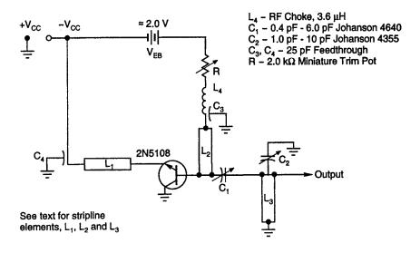
Fig. 6.24 A 1 W, 1 GHz microwave oscillator. Because geometric shapes and dimensions are involved, it often requires a practised eye to discern the equivalent electrical circuit of microwave oscillators
