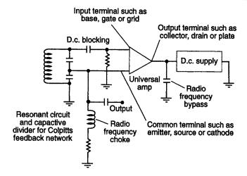
**Fig. 2.29** A basic Colpitts oscillator shown with a three-terminal amplifying device. The implication of such a schematic diagram is that a wide variety of active devices can be employed in the circuit. The triangle is, accordingly, the symbol of the so-called universal amplifier
