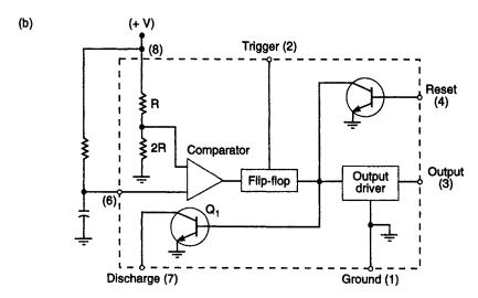
Fig. 5.15 Audio oscillator using the NE555 timer IC. a, Circuit of oscillator suitable for code practice and as a general purpose source of audio frequency test voltage. b, Simplified block diagram of the internal circuitry of the NE555
