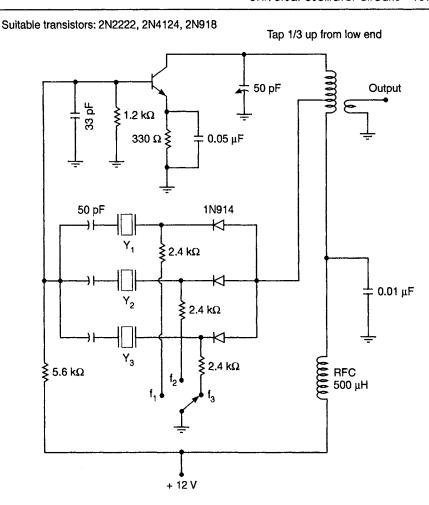
Fig. 5.10 Example of diode switching of crystals. In the above circuit, the three overtone crystals are in the vicinity of 48 MHz. Selection of a frequency should be accompanied by resonating the output tank circuit
