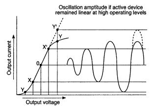
**Fig. 3.14** Limiting action in a Class-A oscillator. Because all active devices depart from linearity at low and high operating levels, equal increments of voltage produce equal increments of current over a restricted amplitude range
