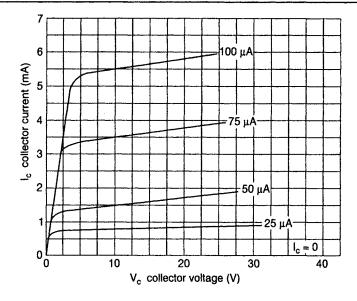
**Fig. 2.1** Common-emitter output characteristics of a typical npn transistor. This is probably the most often used format in oscillator circuits. It tends to provide a reasonable balance of such features as power gain, input impedance, temperature stability and d.c. feed convenience. A small unbypassed resistance connected in the emitter lead will often improve the waveshape of the oscillation
