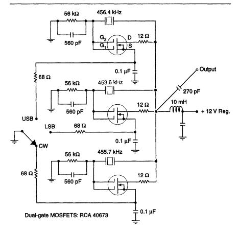
Fig. 5.2 Example of dual-gate MOSFETS in triple BFO arrangement. Each oscillator is a Pierce circuit. By connecting the two gates together, the operation resembles that of JFETs
