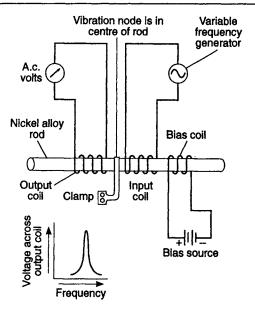
Fig. 1.35 The magnetostrictive oscillating element
