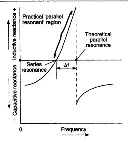
Fig. 1.29 A closer look at the operating conditions of crystals in practical oscillators. Crystals which are spoken of as operating in the 'parallel resonance' mode actually oscillate in a frequency region in which they appear as an inductive reactance
