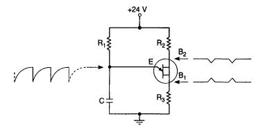
Fig. 4.23 Unijunction transistor relaxation oscillator
