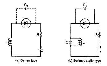
Fig. 3.3 Tunnel-diode sine-wave oscillators
