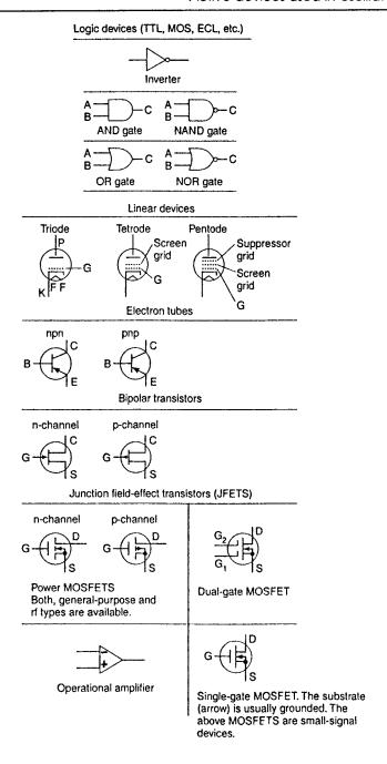
Fig. 2.28 Active devices that can be used in oscillator circuits. The linear devices are readily usable in common oscillators such as the Colpitts of Fig. 2.29. Logic gates are also often used in various oscillator circuits
