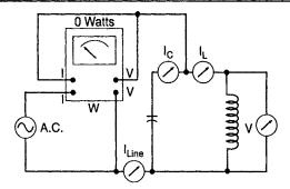
Fig. 1.14 Parallel LC tank circuit for use with Charts 1.1, 1.2 and 1.3
