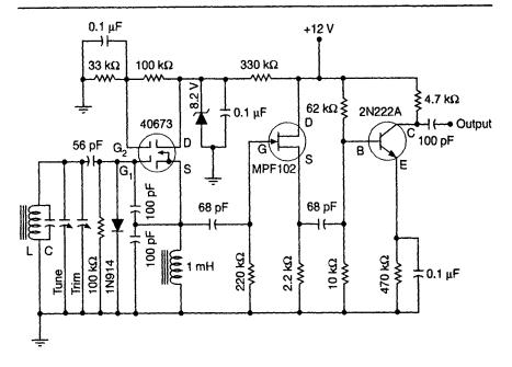
A basic VFO circuit. Select L and C for desired frequency-range. Good performance is readily attainable from 3 to 8 MHz. For many purposes, the TUNE capacitor can be a 100 pF air-variable type. A 25 pF ceramic type should suffice for the TRIM capacitor. Parameter values shown are for sure-fire operation. Modifications may be required for optimum frequency stability
