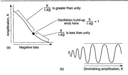
The amplitude-limiting action of automatic bias in an oscillator. a. Amplification as a function of the negative input bias. b, Amplitude limiting caused by oscillation-produced bias. This type of limiting can occur in tube circuits, but not in solid-state oscillators
