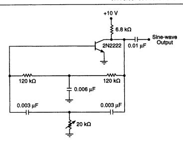
Fig. 5.3 A single-transistor parallel-T oscillator. The natural harmonic discrimination of the T network results in a very low distortion sinusoidal output. The T values shown yield an oscillation frequency of approximately 1 kHz
