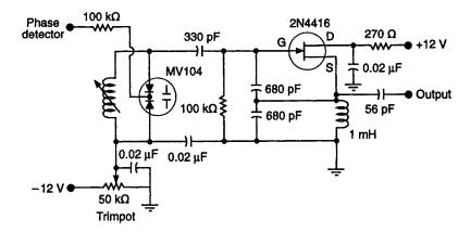
**Fig. 6.11** Voltage-controlled oscillator suitable for use in a phase-locked loop. Note the double varactor in the tuned circuit. Select slug-tuned inductor for the 3 MHz to 8 MHz region. (Much higher frequencies can be designed for with a bit of experimentation and care.) The trimpot provides the mid-operating bias for the varactors
