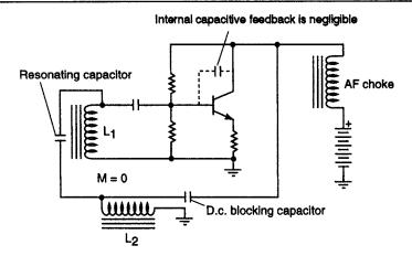
The Type-3 Hartley oscillator. Schematically the same as Fig. 4.2, this Hartley circuit, because of the low oscillation frequency, does not have sufficient collector-base capacitance to cause oscillation. Despite the lack of inductive coupling between output and input, this circuit does oscillate!
