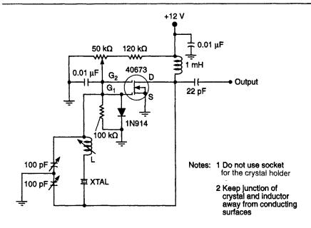
A basic VXO circuit. Derived from a Pierce oscillator, this VXO is capable of exceptionally wide frequency 'pulling'. It should be used with buffer amplifiers such as previously shown with the VFO. The slug-tuned inductor, L, should be selected for either a 7 MHz or a 3.5 MHz crystal. Adjust all variable elements for optimum pulling of the crystal frequency
