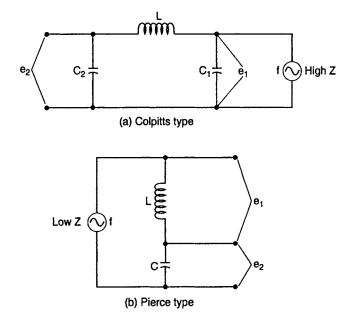
Fig. 1.42 Additional LC networks that produce phase inversion
