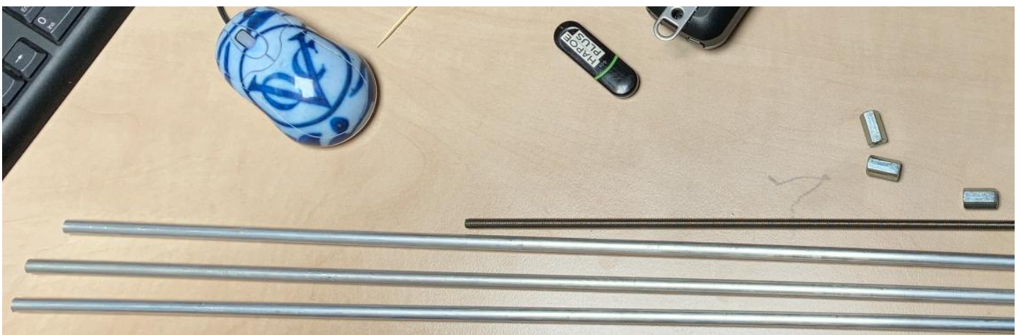
The three aluminium tubes and the CRES threaded end. Plus the three M6 nuts with the larger body.
