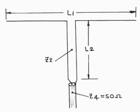
In my analysis of the G5RV configuration using both the Smith chart and my own computer program written in the early 1980s (and more recently using EZNEC) I always called the antenna proper L1 while the "series section matching transformer", that length of transmission line hanging down from its centre, is called L2 and its characteristic impedance is Z2. These details are illustrated in Fig 1.
