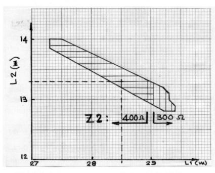
Fig 2 also shows the sensitivity of the multiband match to the value of Z2. It was clear from the analysis that 400 ohms was about optimum, though Z2 = 300 ohms is marginally better for the longest lengths of L1. If values of L1 and L2 close to the extremities within Fig 2 are chosen, the effect is to narrow the bandwidth over which matching will occur in some of the HF bands.
