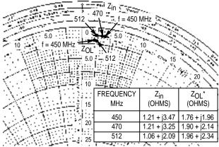
$Z_{OL}^*$  = Conjugate of the optimum load impedance into which the device output operates at a given output power, voltage and frequency.
