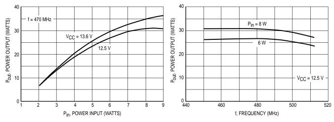
Figure 2. Power Output versus Power Input
