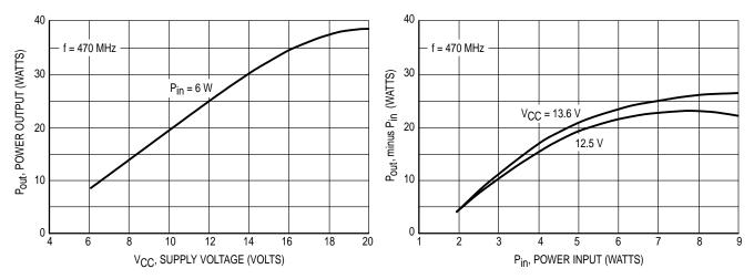
Figure 4. Power Output versus Supply Voltage
