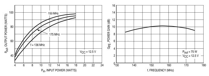
Figure 2. Output Power versus Input Power
