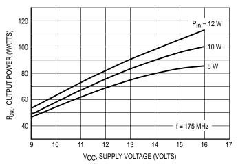
Figure 6. Output Power versus Supply Voltage
