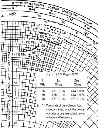
Figure 7. Series Equivalent Impedances
