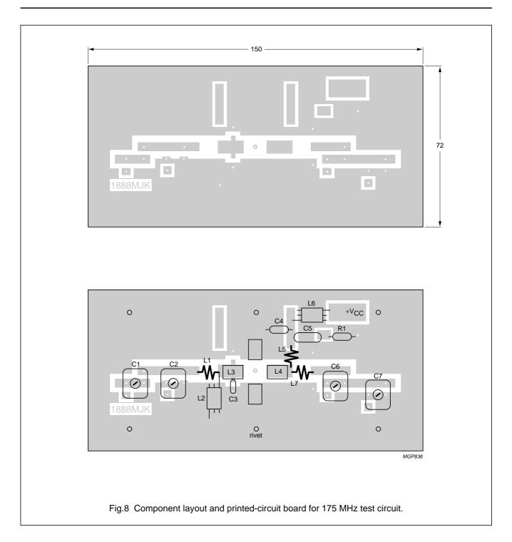
The circuit and the components are situated on one side of the epoxy fibre-glass board, the other side being fully metallized to serve as earth. Earth connections are made by means of hollow rivets, whilst under the emitter leads Cu straps are used for a direct contact between upper and lower sheets.
