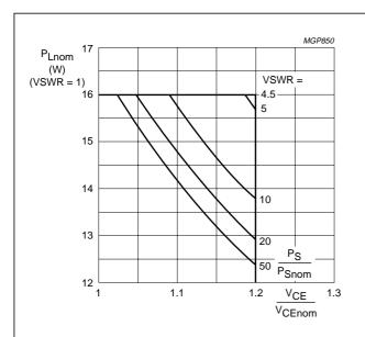
$$\begin{split} & \text{Fig.11} \quad \text{R.F. SOAR (short-time operation during } \\ & \quad \text{mismatch); } f = 175 \text{ MHz; } T_h = 70 \text{ °C;} \\ & \quad \text{R}_{\text{th mb-h}} = 0,45 \text{ K/W;} \\ & \quad \text{V}_{\text{CEnom}} = 13,5 \text{ V or } 12,5 \text{ V;} \\ & \quad \text{P}_{\text{S}} = \text{P}_{\text{Snom}} \text{ at V}_{\text{CEnom}} \text{ and VSWR} = 1. \end{split}$$
