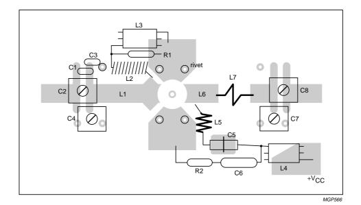
The circuit and the components are situated on one side of the PTFE fibre-glass board, the other side being fully metallized to serve as earth. Earth connections are made by means of hollow rivets.
