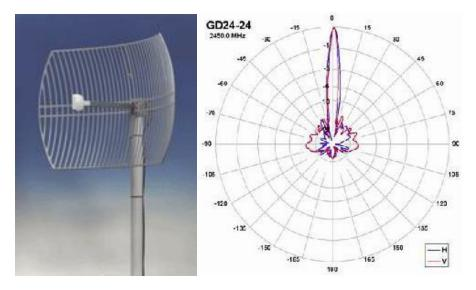
Figure 29 Liard 24dBi Grid Parabolic Dish Antenna and Radiation pattern [38]
