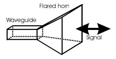
Figure 14 Example of a Horn Antenna [22]
