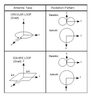
Figure 13 Radiation Pattern of a Small Circular and Rectangular Antenna [20]
