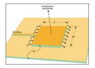
Figure 18 Basic Patch Antenna Design [28]
