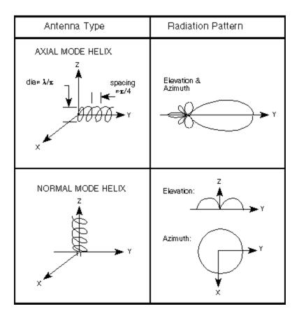
Figure 11 Radiation Pattern of Helix Antenna [18]
