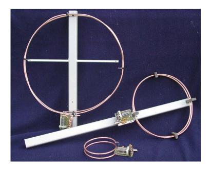
Figure 12 Loop Antenna Example [19]
