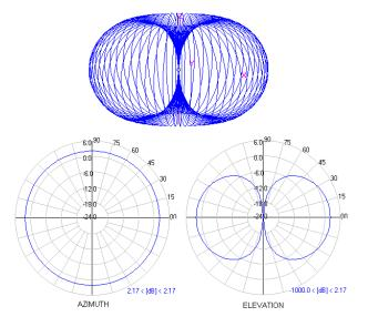
Figure 5 Dipole Radiation Pattern [12]
