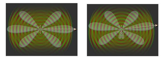
Figure 24 Left- Array Element with same phase; Right - array element on bottom with 10 degree phase shift [33]
