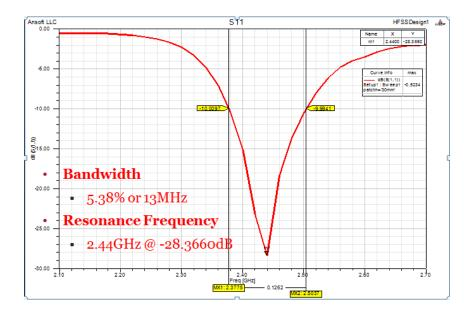
Figure 33 Simulated Reflection Coefficient with 30x30mm Patch
