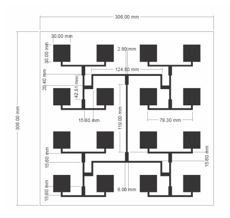
Figure 32 Schematic of Microstrip Antenna Array
