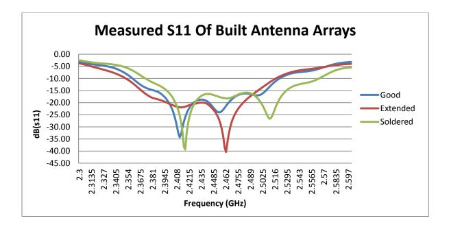
Figure 36 Measured S11 of Antenna Arrays
