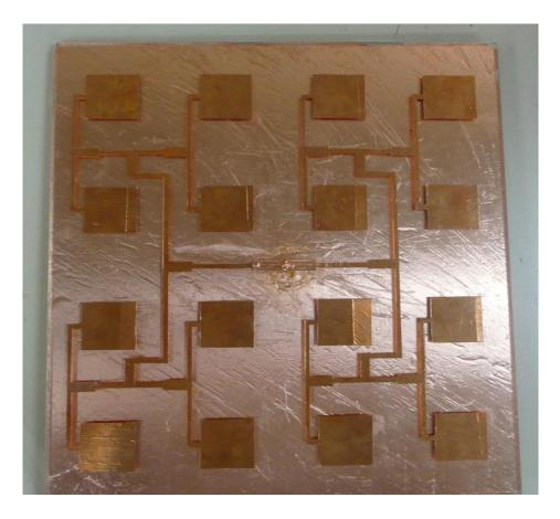
Figure 35 Constructed Antenna Array with 30x34mm Rectangular Patches
