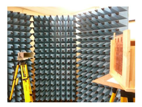
Figure 38 Antenna Radiation Measurement Setup
