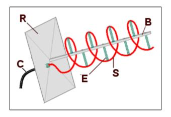
Figure 10 Basic Helix Antenna Configuration [17]
