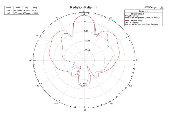
Figure 34 Radiation Pattern of Simulated Patch Antenna Array
