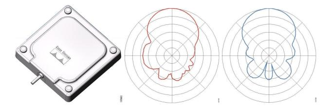
Figure 27 CISCO AIR-ANT5195P-R Aironet 9.5-dBi Patch Antenna and Radiation Patter (Red-Vertical, Blue-horizontal) [36]
