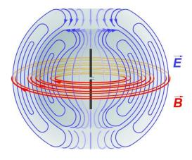
Figure 4 Dipole Antenna and Radiation Pattern [11]
