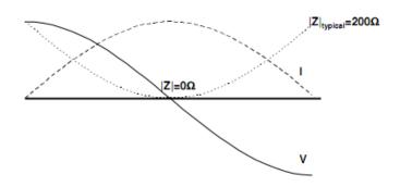
Figure 19 Voltage and Current Distribution of Patch Antenna [29]
