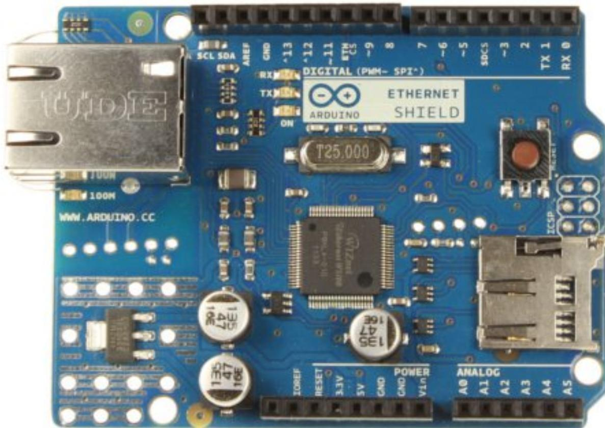
FIGURE VIII.1.2. – Le shield Ethernet Arduino - (CC-BY, [arduino.cc](http://arduino.cc) [↗](#))
