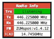
2. If you transmit and the modem receives it, the Radio Info TRX section will be green and will display "RX [mode]." If the modem receives a transmission from someone else and transmits it to your radio, the Radio Info TRX section will be red and will display "TX [mode]" (if the mode is DMR, it also displays the time slot). While in the TX status, you can't break in with your own transmission.
