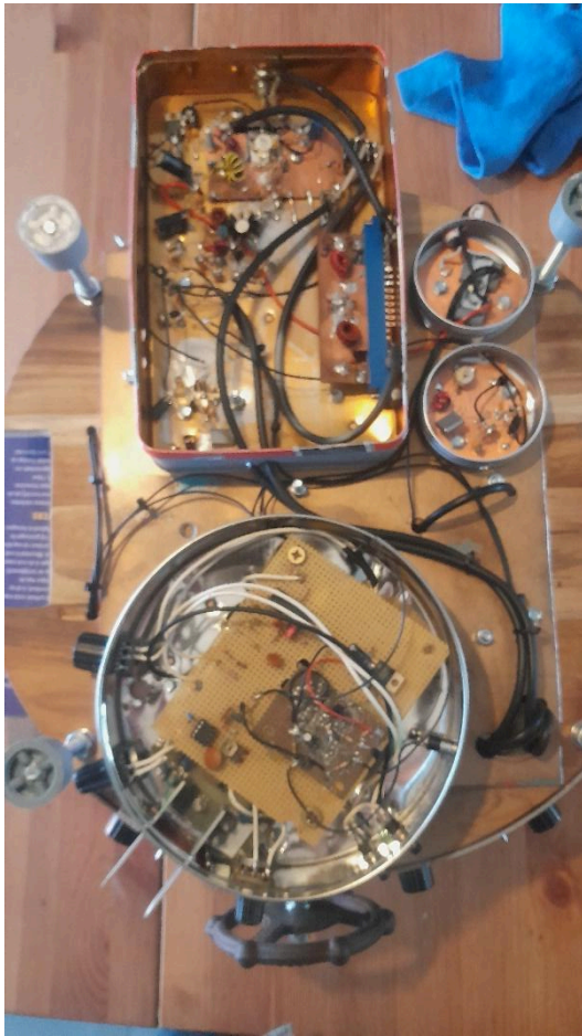
Keyer and linear with plug-in low pass filters.
