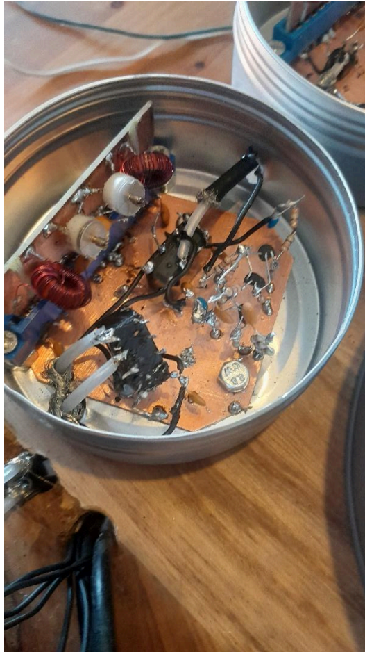
The plug-in band pass, T/R relay and RF amplifier.
