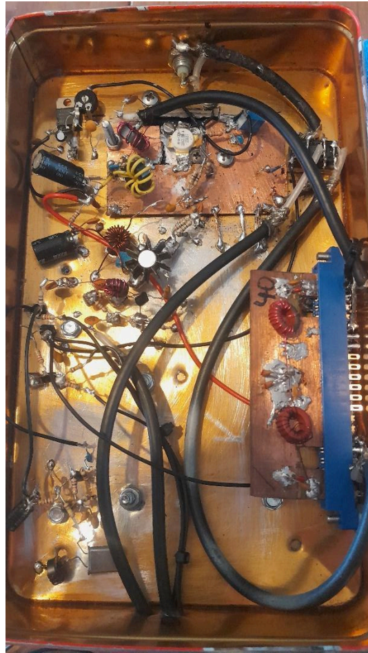
Keyer and linear with plug-in low pass filters.
