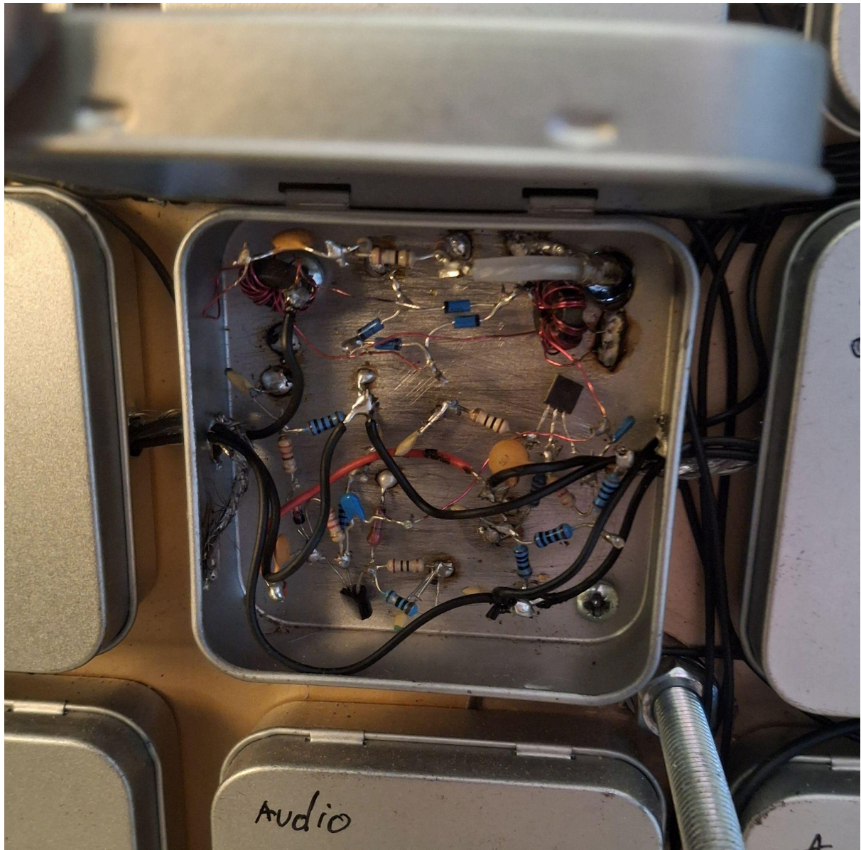
Mixer 1, mine are not as beautifully built but beauty does not matter. The 4 diodes are out in the breeze.
