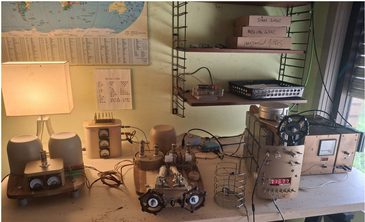
From left to right, tube power supply, solid state power supply, tube regenerative receiver, SSB transceiver and linear. All the Bosses in a neat row.
