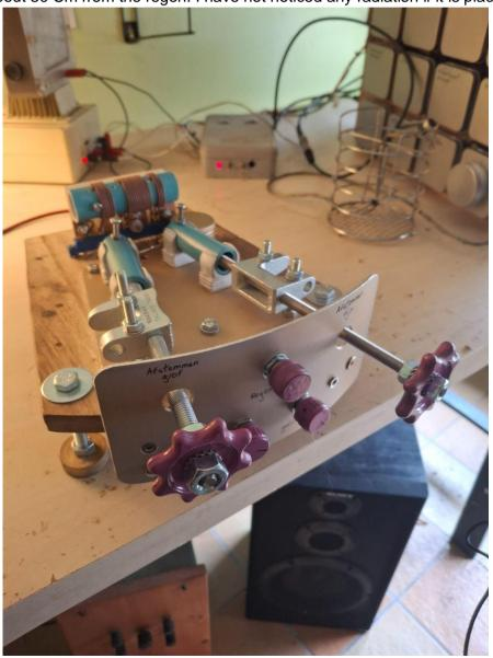
The homebrew capacitors are basically a threaded rod that are being driven in or out a metal tube. One is M10 in a tube that is about 12mm. This is the coarse tuning and is probably about 35 pF. The other one is a M8 rod in a 17 mm tube. Probably around 10pF. The rods are driven through a M10 and M8 steel beam clamp. These provide gear reduction. About 1/40.
