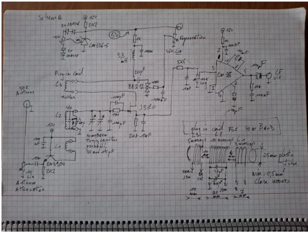
Differences with the original circuit? I used a LM386 for the audio amplification and a J310 for the regenerative oscillator. The HF amplifier is done with a 2N3904. After the set worked with a classic tuning capacitor for the regeneration I swapped it for a BB212 varicap. The coil is plug-in. So far only a 40M band coil is made. I will probably never make coils for other bands as the 40M band is my favorite.
