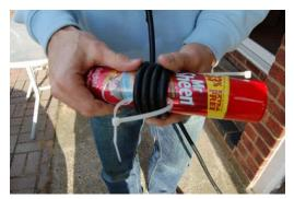
Once you have the desired number of turns on the can, join the end sections of the cable ties and pull them tight in order the choke is firm and will not go out of shape or remove itself from the loop.
