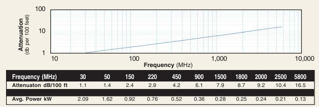
Calculate Attenuation = (0.191930) • √FMHz + (0.000330) • FMHz (interactive calculator available at http://www.timesmicrowave.com/cable\_calculators) Attenuation: VSWR=1.0; Ambient = +25°C (77°F) Power: VSWR=1.0; Ambient = +40°C; Inner Conductor = 100°C (212°F); Sea Level; dry air; atmospheric pressure; no solar loading
