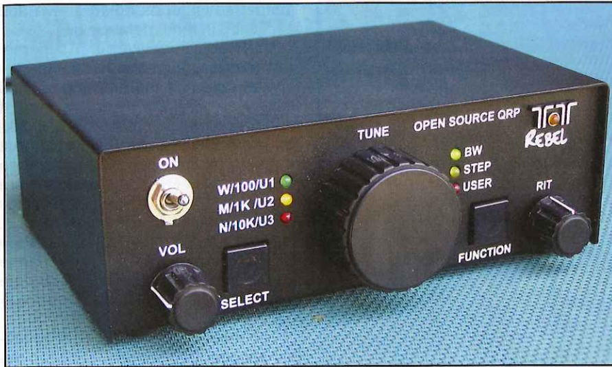
Photo C— The Ten-Tec Rebel is something new in ham radio gear—an open-source, factory-built QRP transceiver. See text for details.
