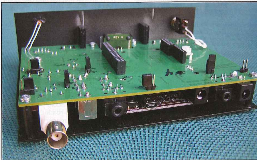
Photo D— Backside view of the Ten-Tec Rebel. The USB port is attached to the Arduino board. Also note jack for key or external keyer output.
