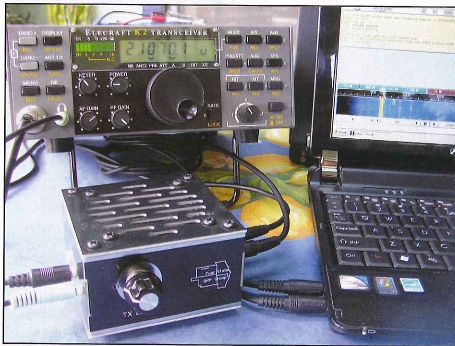
Photo E— The Four State 4S-Link set up for a PSK-31 session.
