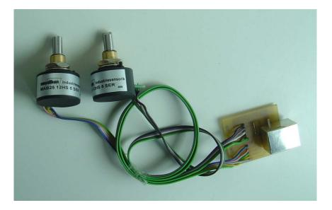
For Az/El encoder connection you additionally need the small splitter PCB and a 8 pin LAN connector.
