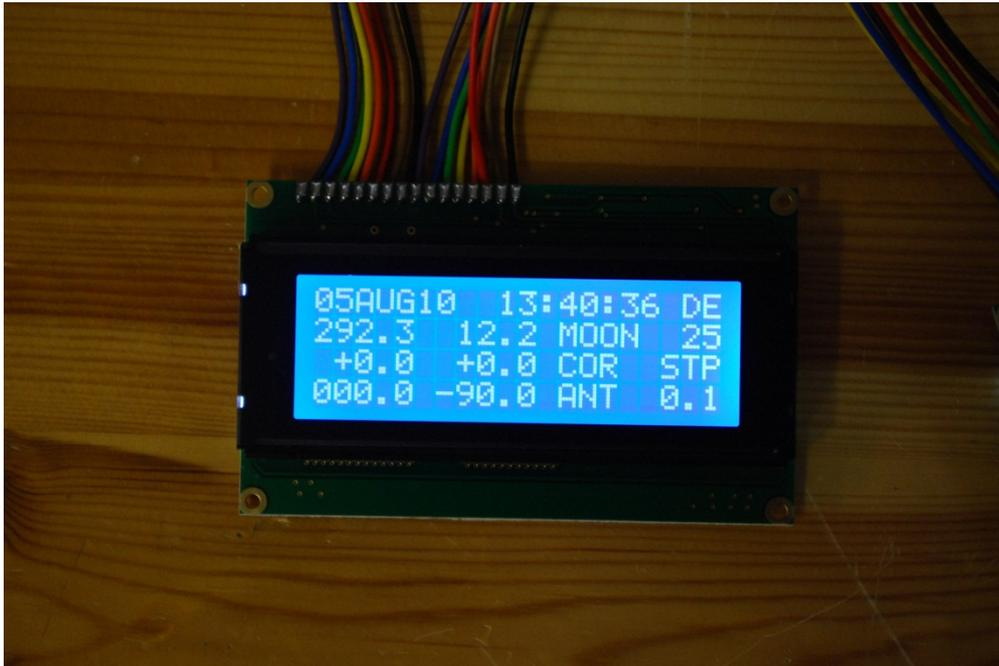
NOTE: The antenna in this example show AZ=000.0 and EL=-90.0 because the interface board and the encoders are not connected during the photo.
