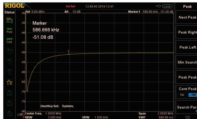
Figure 6 – Low Frequency Response of Sampler
