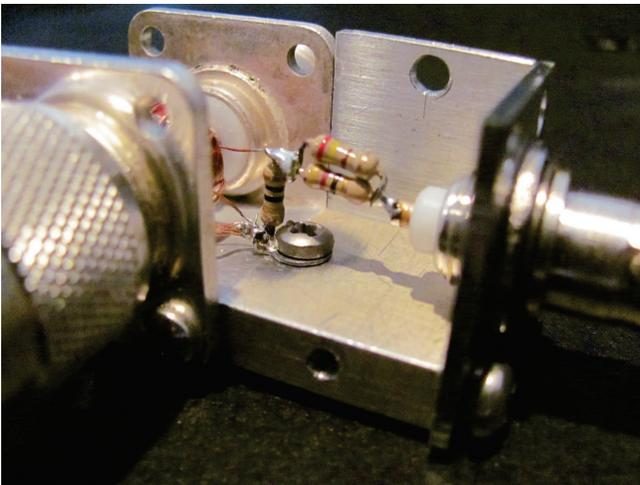
The transformer is constructed by winding 32 turns of 30AWG enameled magnet wire on a Micrometals 44-2 powdered iron core. This core can be ordered online from Amidon Corporation. Wind a single layer of wire on the core, taking reasonable care to leave a little space between each winding. This will help minimize the distributed capacitance of the transformer.
