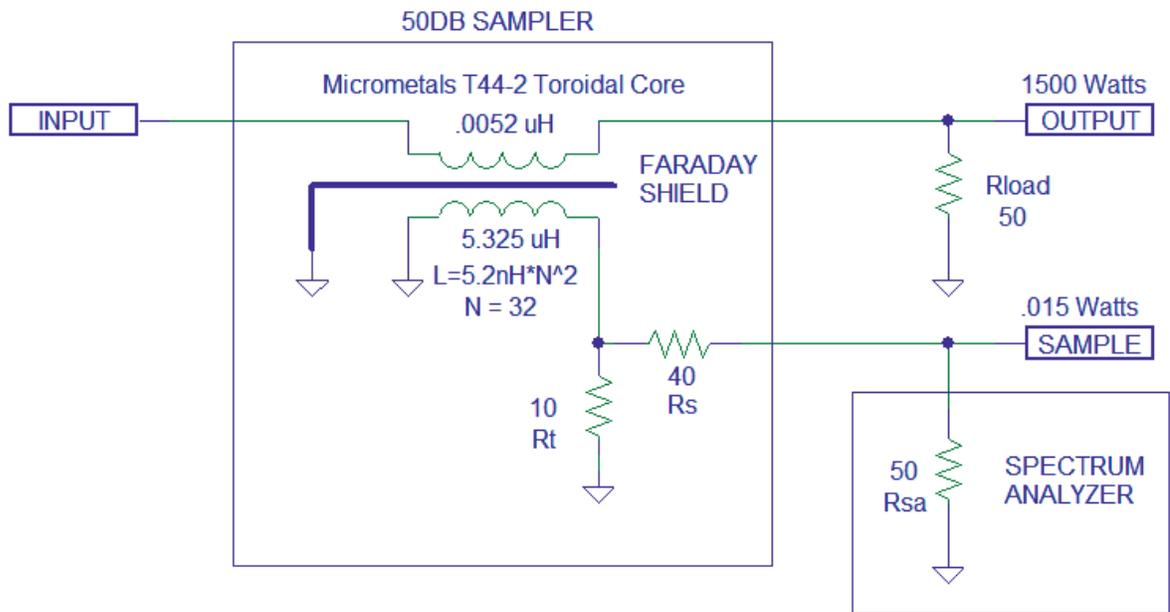
Figure 1 – Schematic Diagram
