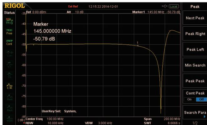
Figure 5 – High Frequency Response of Sampler
