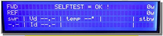
Self Test complete and all tested circuits working properly
