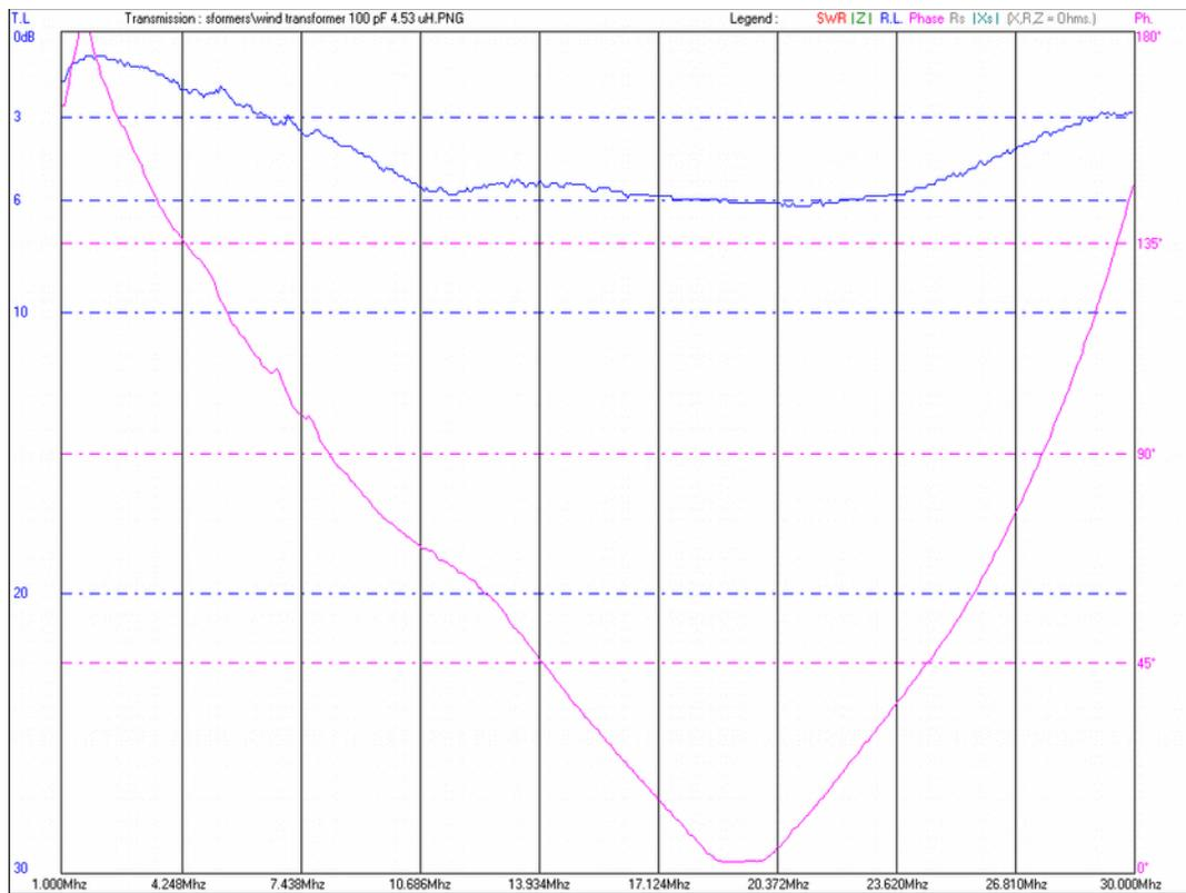
Back-to-back transformer test with 4.5  $\mu\text{H}$  of inductance in series between the two secondaries of the transformers. Resonance occurs at about 30 MHz with about 1.5 dB loss per transformer.
