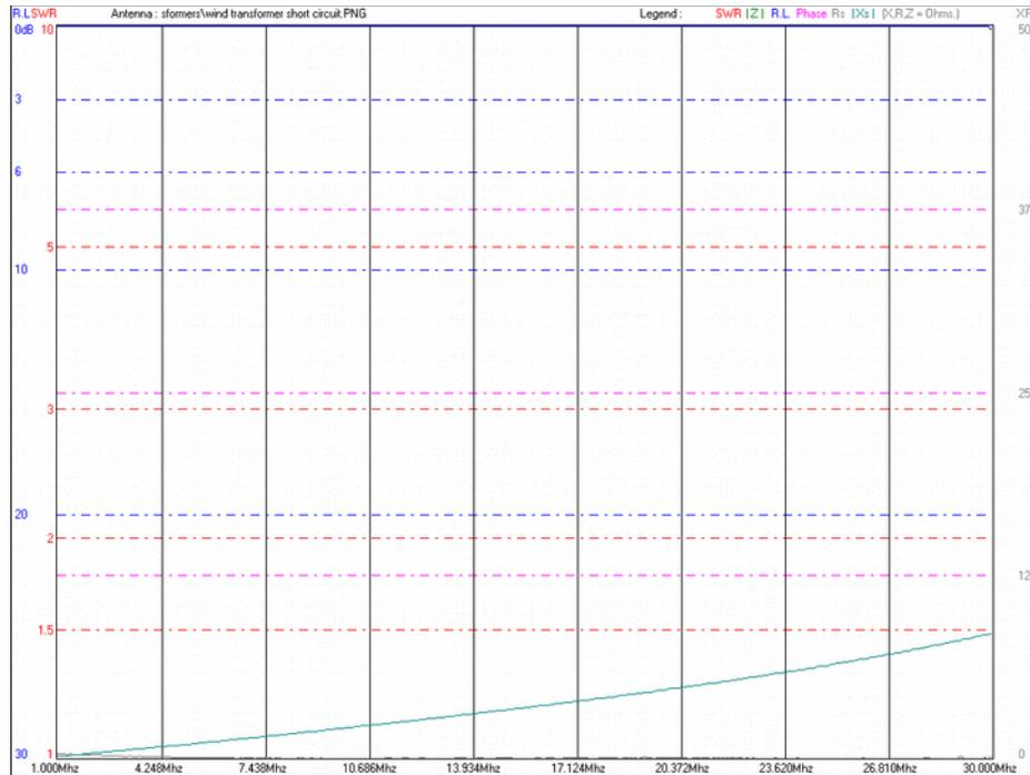
Short circuit reactance of the transformer. To calculate the leakage inductance, at a frequency well below the self-resonance frequency, such  $f = 10$  MHz, observe the reactance, which in this case is approximately  $X = 20 \Omega$ . Then the leakage inductance  $L_I = X/(2\pi f)$  or approximately  $0.3 \mu\text{H}$ .
