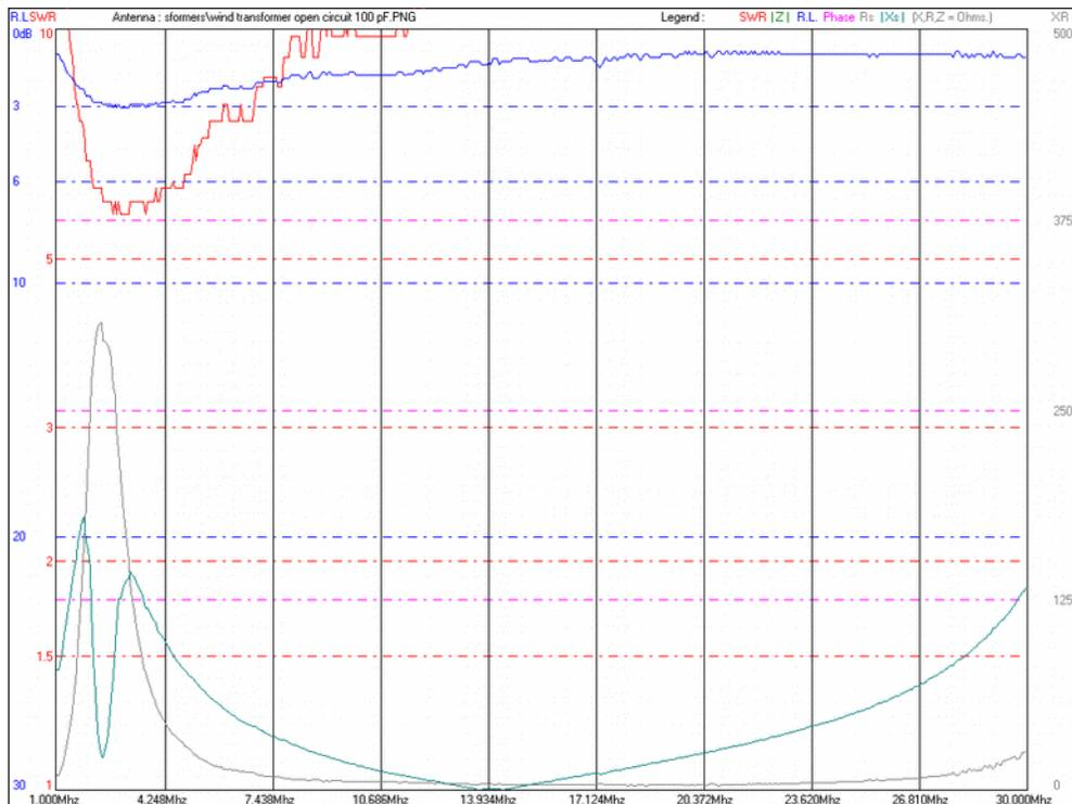
Open circuit reactance of the transformer with  $C_p = 100 \text{ pF}$  across the primary. The new resonant frequency is  $f = [8\pi^2 (C_s N_s^2 / N_p^2 + C_p) L_I]^{-0.5}$  or 13.6 MHz as predicted.
