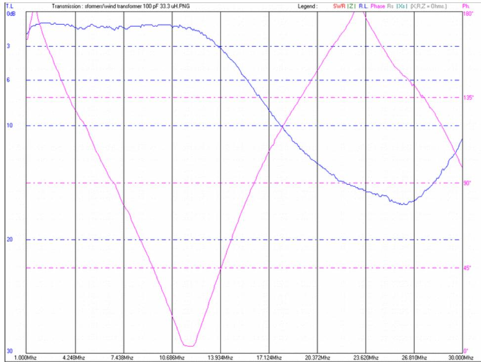
Back-to-back transformer test with 33.3  $\mu\text{H}$  of inductance in series between the two secondaries of the transformers. Resonance occurs at about 10 MHz with about 0.5 dB loss per transformer.
