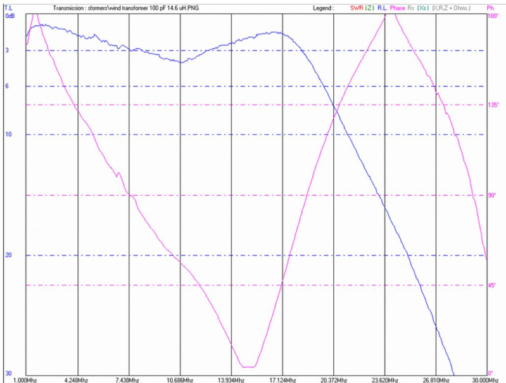
Back-to-back transformer test with 14.6  $\mu\text{H}$  of inductance in series between the two secondaries of the transformers. Resonance occurs at about 16 MHz with about 0.75 dB loss per transformer.
