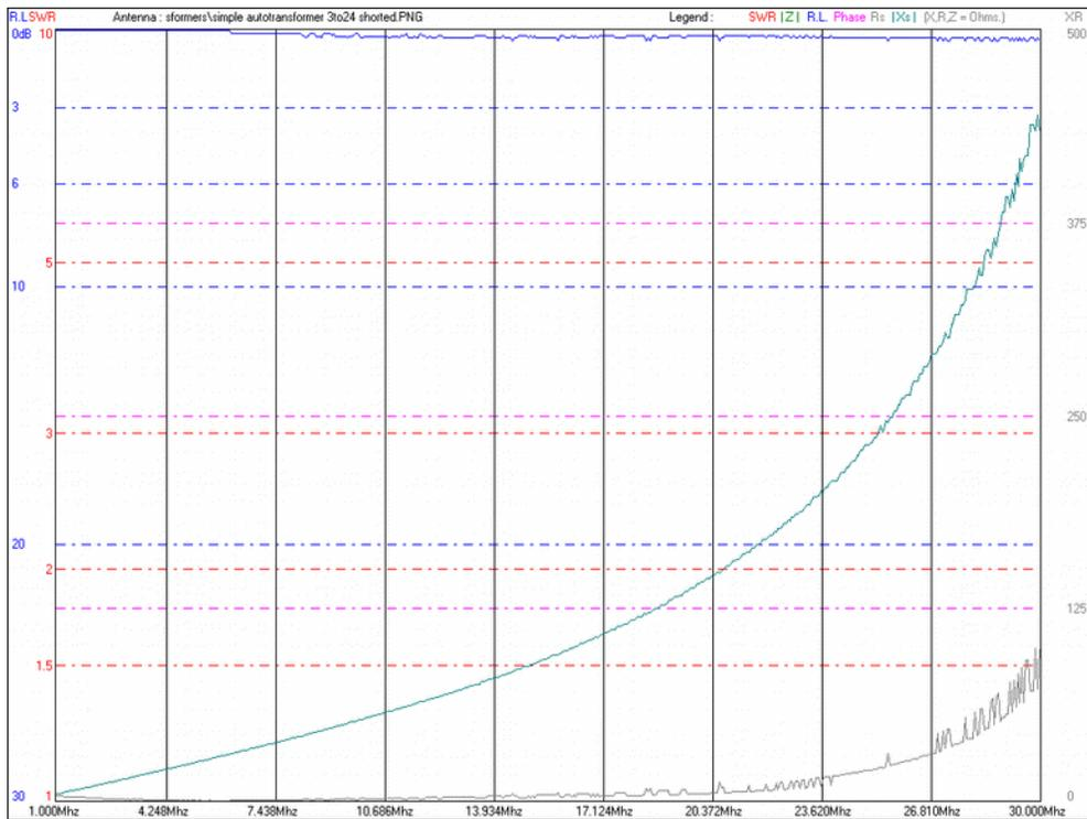
The short circuit test indicates  $57 \Omega$  ohms of impedance at 10.68 MHz which corresponds to  $0.85 \mu\text{H}$  leakage inductance.
