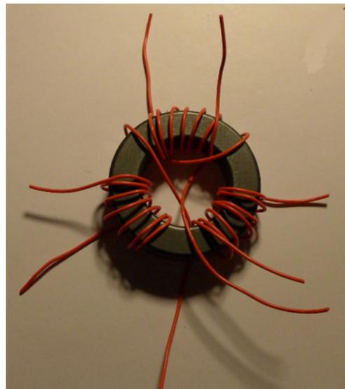
Wrap a fourth wire between the three coils in the same direction
