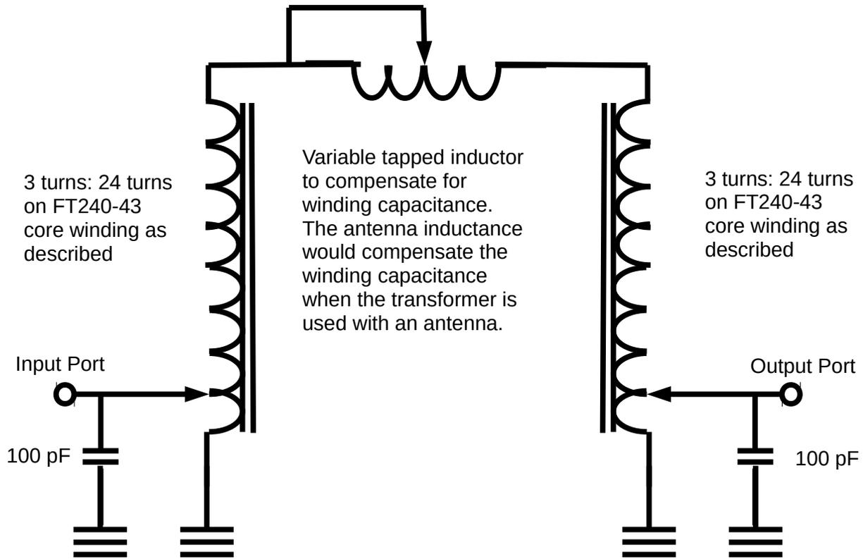
As the inductance between the two transformers is increased, the winding capacitance is resonated at a lower frequency. At the resonant frequency, the winding capacitance is an open circuit and therefore does not degrade the impedance transformation.
