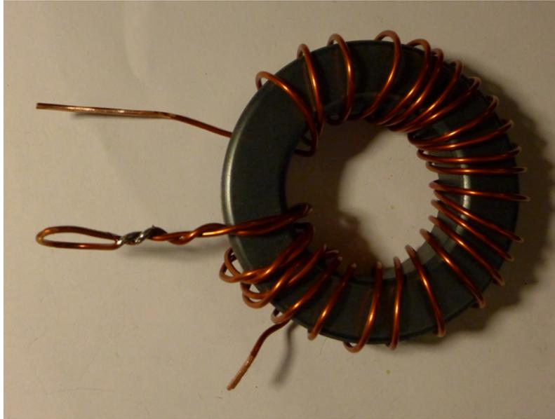
This uses a more conventional winding technique with 3 turns of primary and secondary that are twisted together, and 21 more turns of separated secondary winding.
