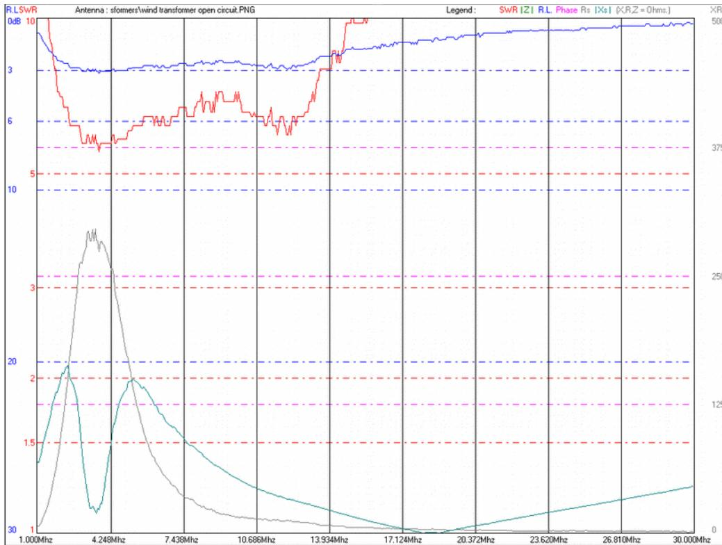
Open circuit reactance of the transformer. With  $L_I = 0.3 \mu\text{H}$  leakage inductance, for series resonance to occur at  $f_R = 18 \text{ MHz}$ , the secondary winding capacitance is  $C_s \approx N_p^2 / (8\pi^2 N_s^2 L_I f^2)$  or 2 pF.
