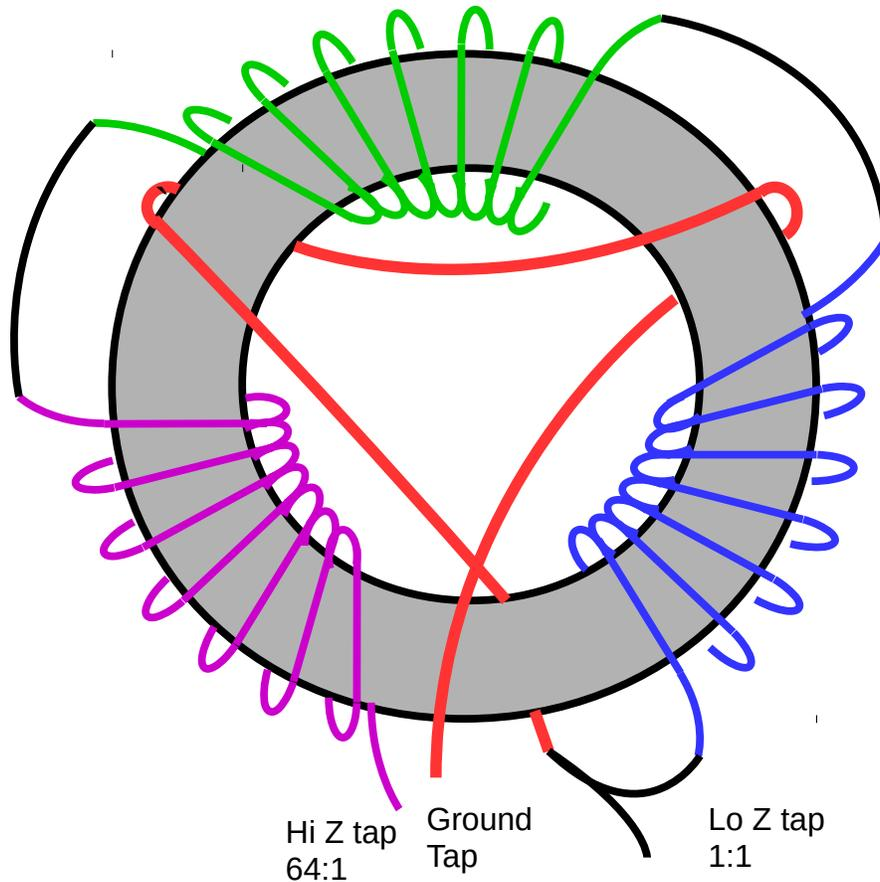
Winding pattern of the 3:24 turn end-fed half-wave transformer.
