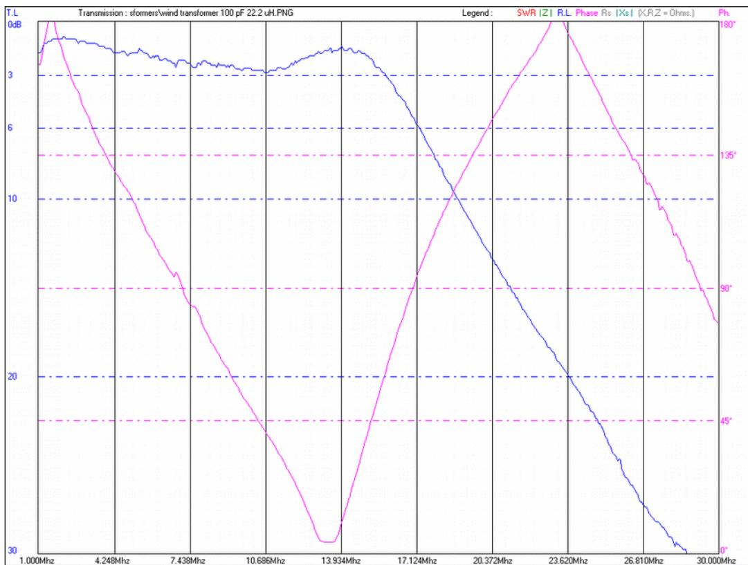
Back-to-back transformer test with 22.2  $\mu\text{H}$  of inductance in series between the two secondaries of the transformers. Resonance occurs at about 14 MHz with about 0.75 dB loss per transformer.
