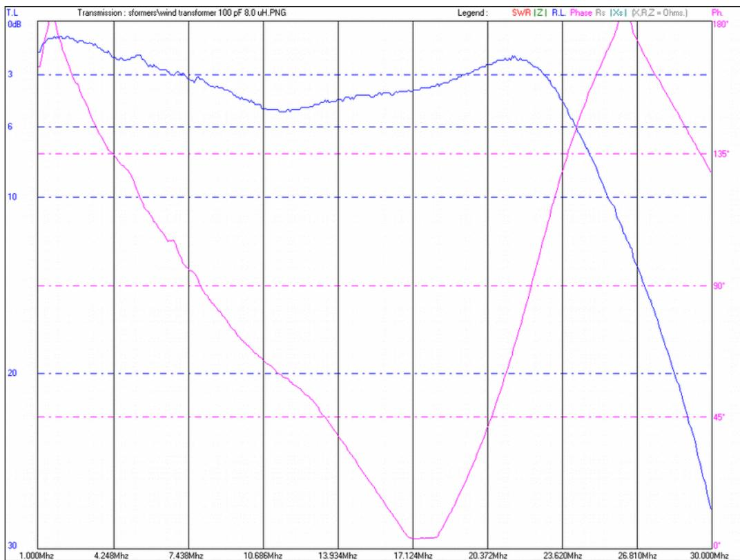
Back-to-back transformer test with 8.0  $\mu\text{H}$  of inductance in series between the two secondaries of the transformers. Resonance occurs at about 22 MHz with about 1 dB loss per transformer.
