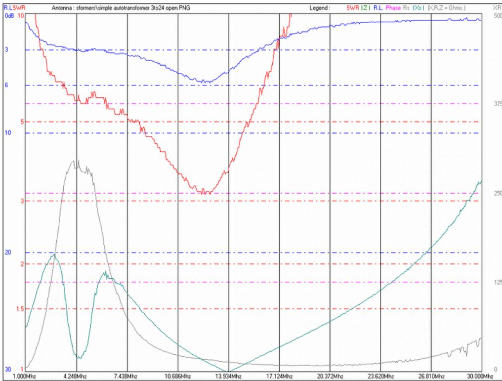
The open circuit test indicates a series self resonance frequency of 13.6 MHz which corresponds to a secondary winding capacitance of 1.26 pF.
