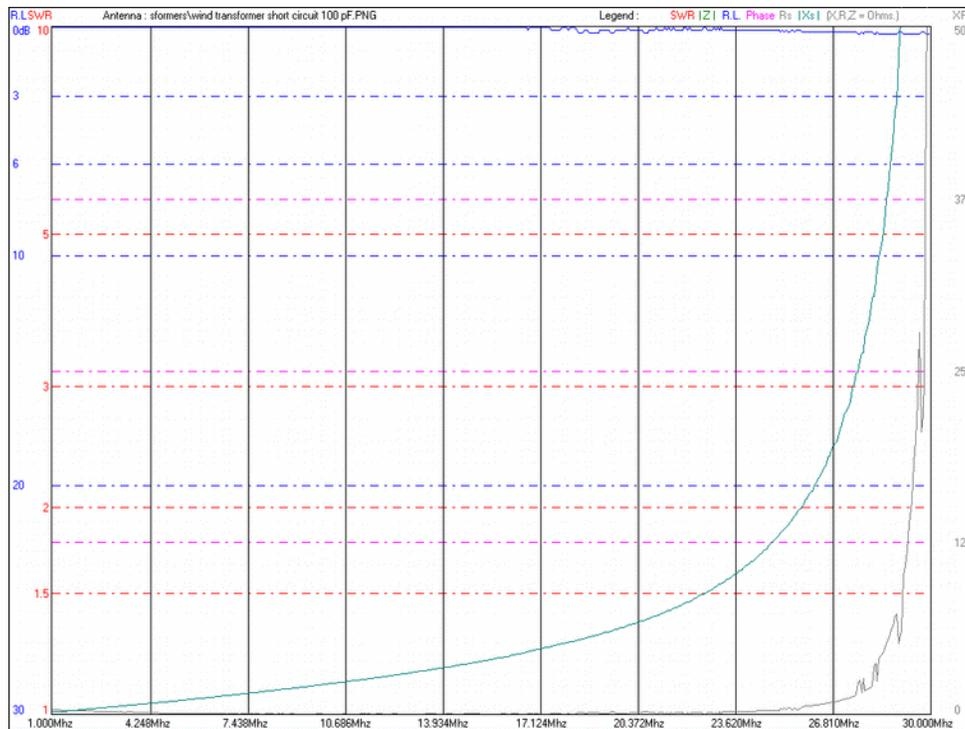
Short circuit reactance of the transformer including a  $100 \text{ pF}$  capacitor across the primary.
