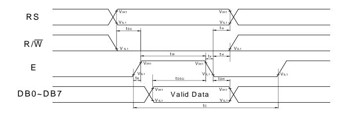
Fig. a Interface timing (data write)
