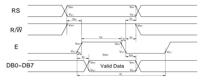
Fig. b Interface timing (data read)
