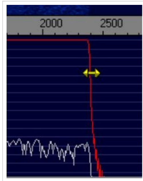
Figure 10 - Dragging the upper passband limit with the mouse
