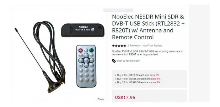
This custom NooElec SDR is a modified DVB-T USB dongle tuned for SDR usage, including upgraded crystal, capacitors and inductors compared to generic devices. Full compatibility with a large array of software packages, such as MATLAB®, HDSDR, SDR Touch, SDR#, Planeplotter--too many to list.
