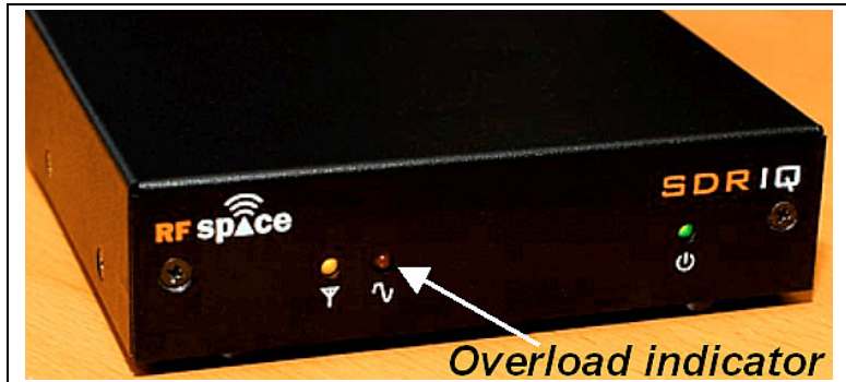
Figure 12: The overload indicator on the front panel of the SDR-IQ
