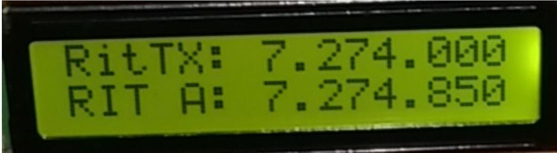
VFO A is in use, and the uBITX will transmit on 7.274.000, and it will receive on 7.274.850
