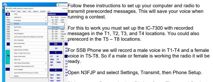
Pick your com Port, and select Rig Interface. (The sound Card option seems to be only if you have audio recordings on the computer instead of the radio.)
