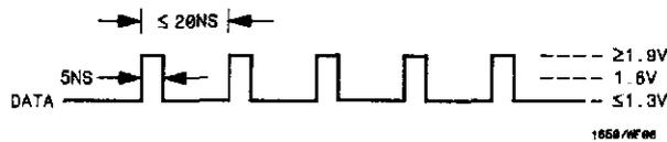
Figure 3-27. Waveform for Glitch Test
