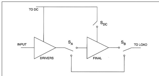
Figure 24 · Stage-bypassing architecture.
