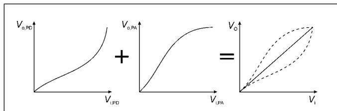
Figure 50 · Amplitude correction by predistortion.
