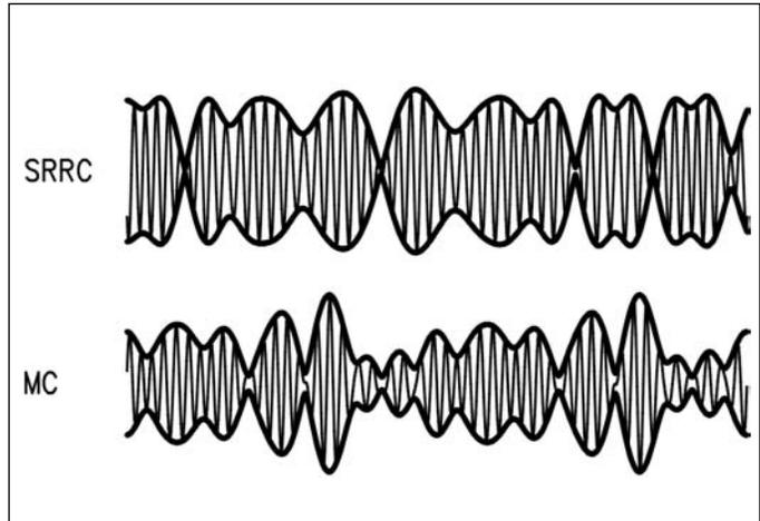
Figure 2 · RF waveforms for SRRC and multicarrier signals.
