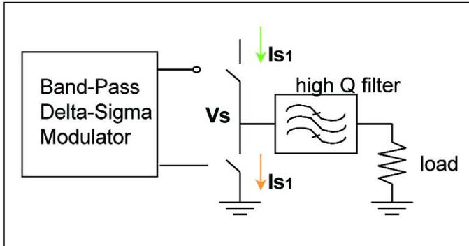
Figure 63 · Delta-sigma modulator.
