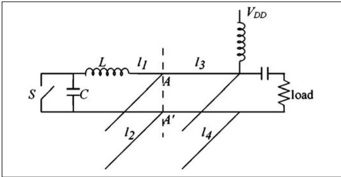
Figure 13 · Idealized microwave class-E PA circuit.
