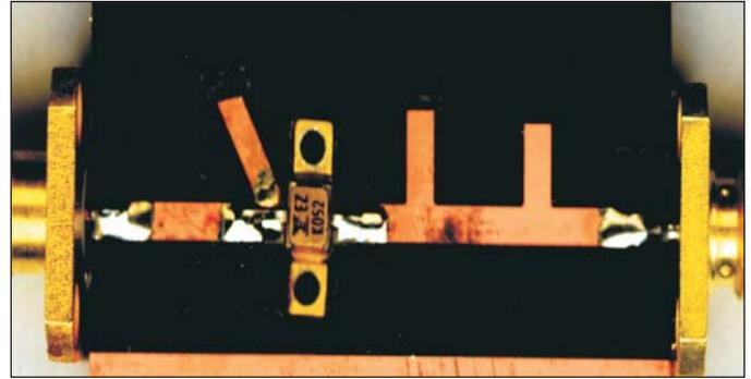
Figure 14 · Example X-band class-E PA.
