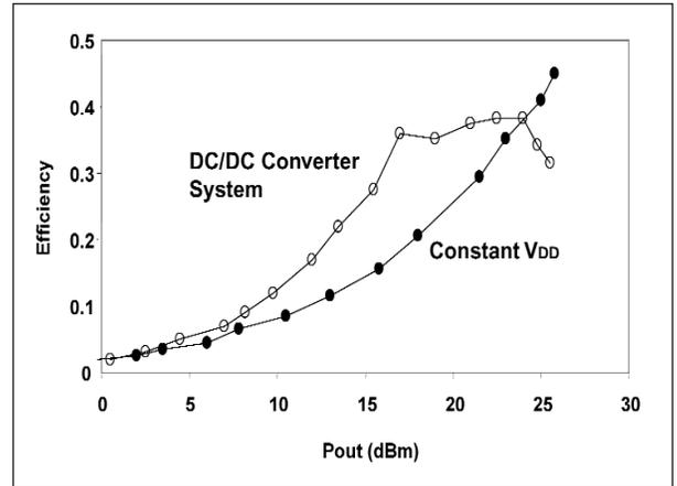
Figure 32 · Efficiency of a GaAs FET envelope-tracking transmitter.
