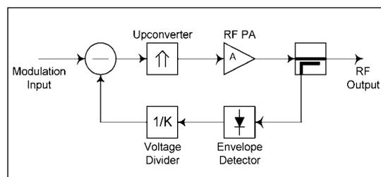
Fig 41 · Envelope feedback applied to a complete transmitter.
