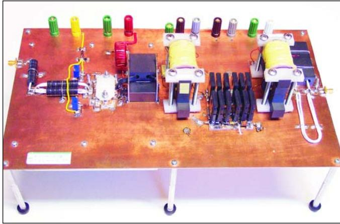
Figure 68 . Electronically tunable class-D PA (courtesy GMRR).
