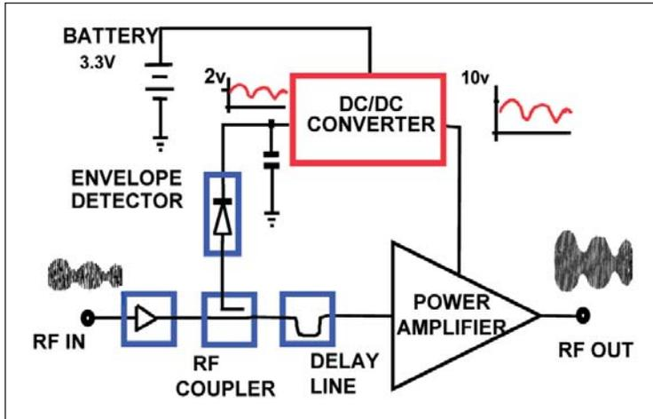
Figure 31 · Envelope-tracking architecture.
