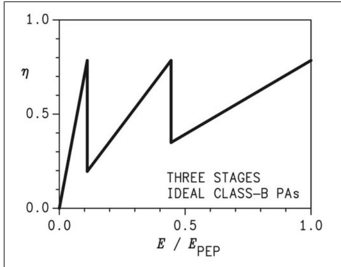
Figure 67 . Instantaneous efficiency of switched PAs.
