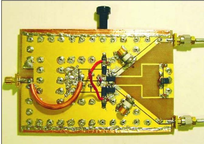
Figure 60 · Current-switching PA for 1 GHz (courtesy UCSD).
