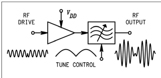
Figure 69 · Load modulation by electronic tuning.
