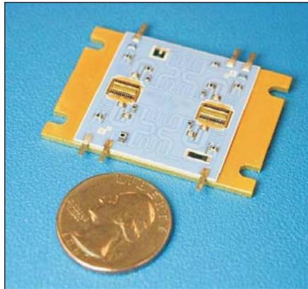
Figure 18 · Thick-film hybrid S-band PA module. (Courtesy UltraRF)
