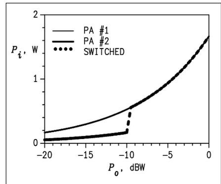
Figure 23 · Power consumption by PAs of different sizes.
