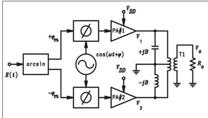
Figure 36 · Chireix-outphasing transmitter.
