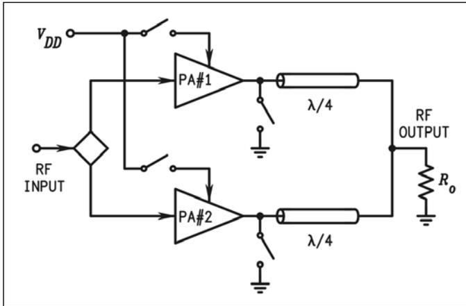
Figure 66 . Switched PAs with quarter-wavelength transmission line combiner.
