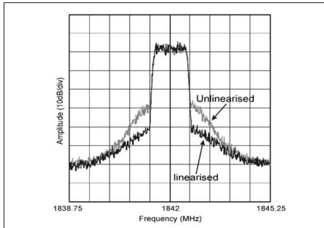
Figure 52 - Linearization by diode-based RF predistorter (courtesy WSI).
