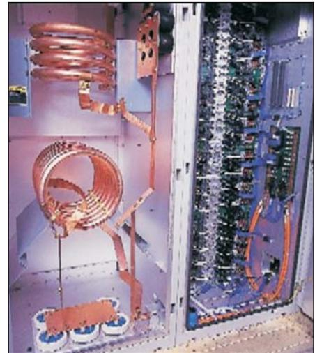
Figure 16 · Output section of a 50-kW AM broadcast transmitter. (Courtesy Harris)
