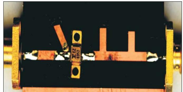
Figure 14 · Example X-band class-E PA.
