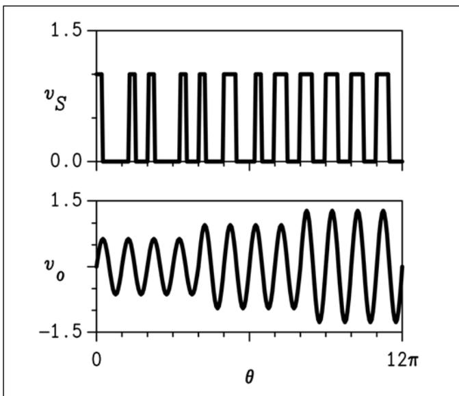
Figure 62 · Delta-sigma modulation.
