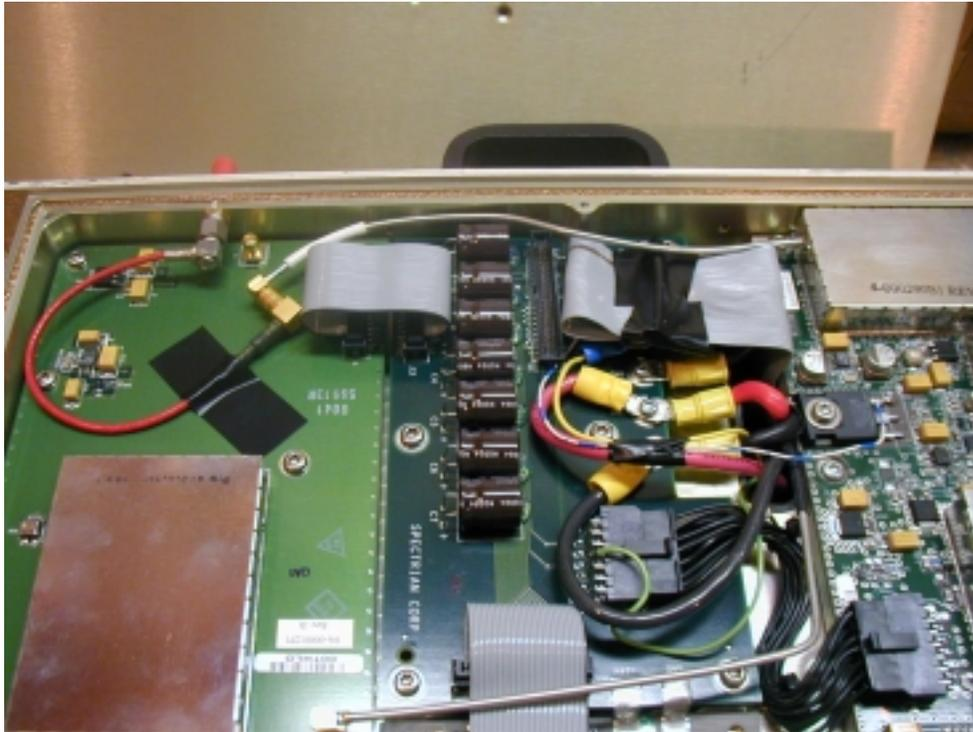
**Figure 4** View of RF input connections (a female-to-female sma bulkhead connector mates with a right-angle sma-male connector on a red jumper cable; the smc-female connector on the other end of that cable mates with the MCX-male connector on the original jumper cable to the RF driver board).
