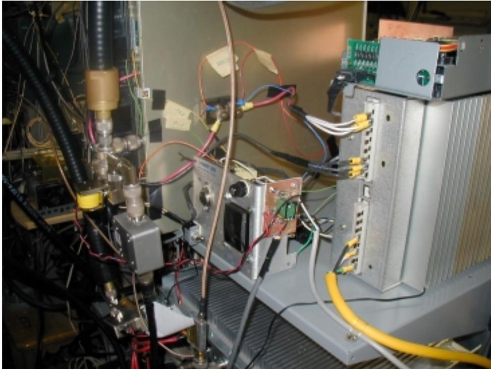
**Figure 6** Rear view of Spectrian amplifier tray, showing transmit/receive relay connection to 7/8" Heliac antenna feed line and low-noise preamp; also shown are the 12 VDC fan power supply and the 26 VDC switcher power supply with 50 amp meter shunt..
