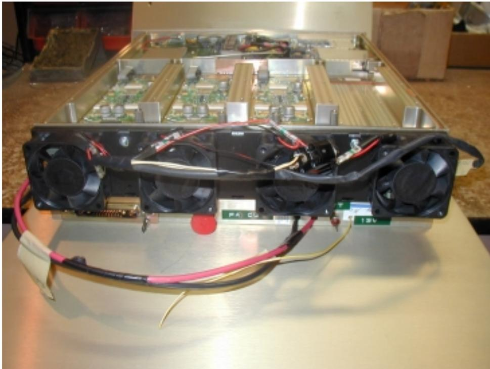
**Figure 1** View of 4 small 12 VDC fans mounted on rear of chassis to push air through the unit for cooling purposes.
