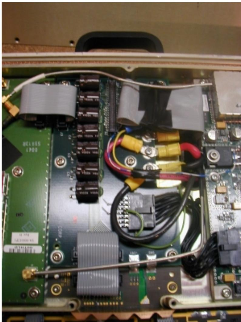
**Figure 5** View of 26 VDC (red) and return (black) cables, blue/white jumper to route 13 VDC to amplifier modules, green wire for PTT control (ground enables the transmitter), and yellow wire for monitoring 13 VDC.
