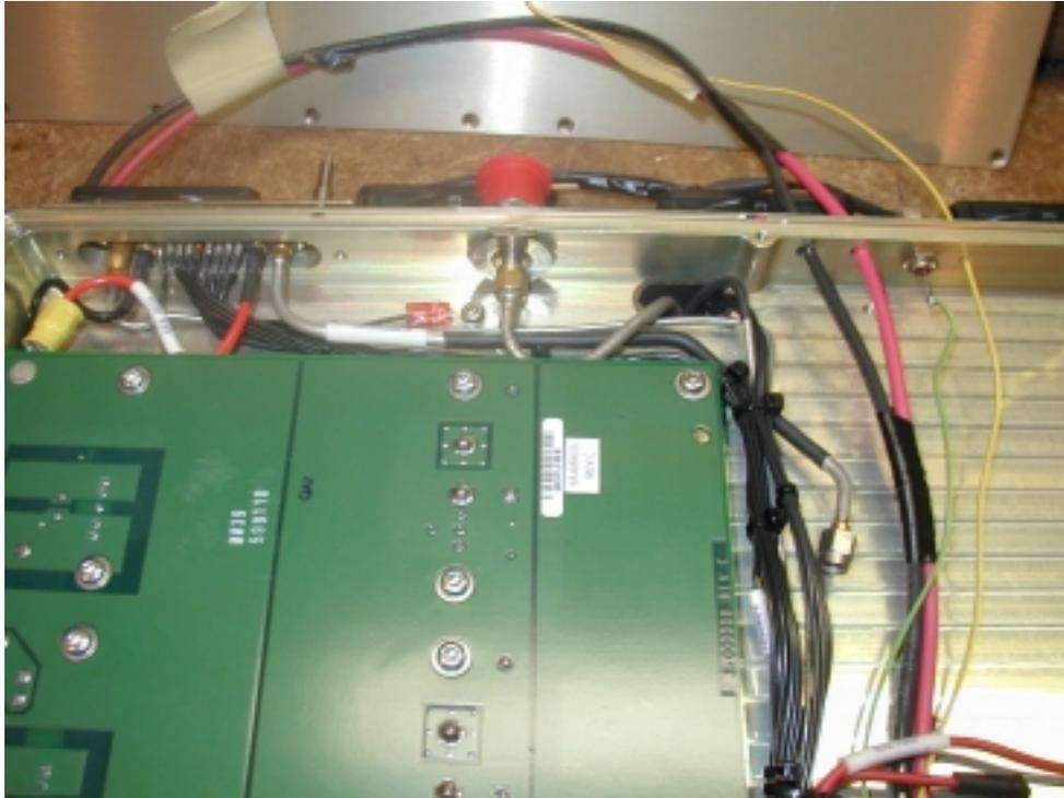
**Figure 3** View of other end of 0.141” semi-rigid cable (an sma-male connector mates with an sma-female to N-female bulkhead adaptor).
