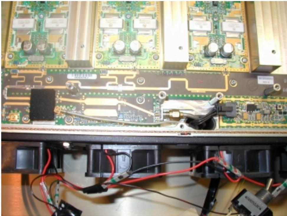
**Figure 2** View of amplifier output to 0.141" semi-rigid cable, sma-male end.
