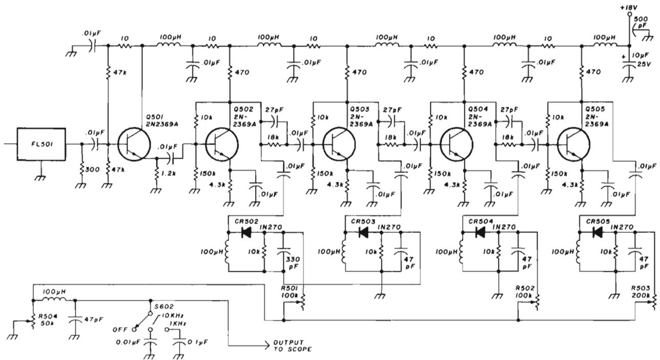
fig. 12. Log amplifier schematic.
