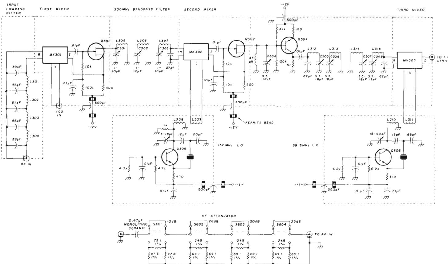
fig. 10. Rf-section schematic. All bipolar transistors are 2N2369As; fets are J309 or J310. Feedthrough caps are 500 pF.
