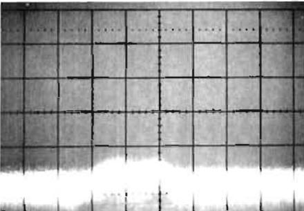
fig. 24. BW 250 kHz. Scan 100 kHz/division and generator frequency about 40 MHz. Increase generator output to see a signal in the noise with the video filter off.
