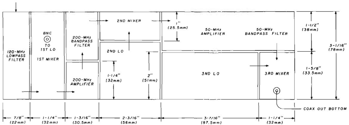
fig. 14. Rf-section dimensions.
