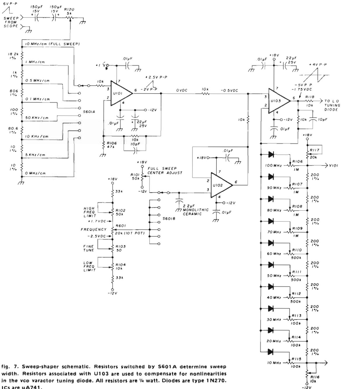
fig. 7. Sweep-shaper schematic. Resistors switched by S601A determine sweep width. Resistors associated with U103 are used to compensate for nonlinearities in the vco varactor tuning diode. All resistors are 1/4 watt. Diodes are type 1N270. ICs are uA741.
