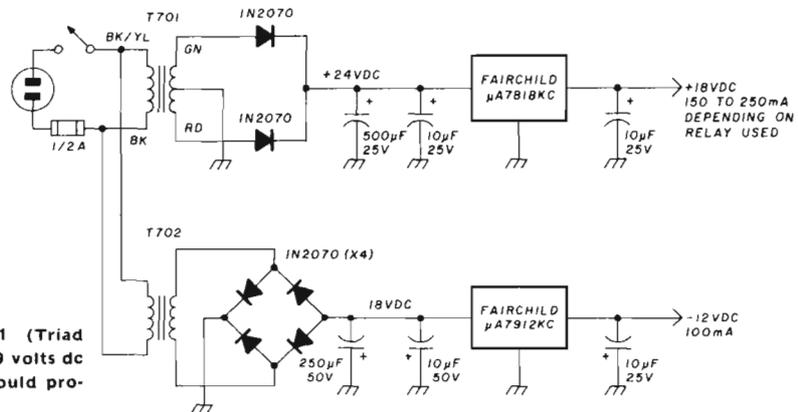
fig. 17. Power-supply schematic. T701 (Triad F90X or equivalent) should provide 23-29 volts dc at approximately 200 mA, and T702 should provide 18-24 volts dc at 100 mA.
