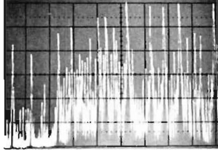
fig. 22. After connecting antenna to inputs, turn BW to 1 kHz and note how stations in the broadcast band can be resolved.
