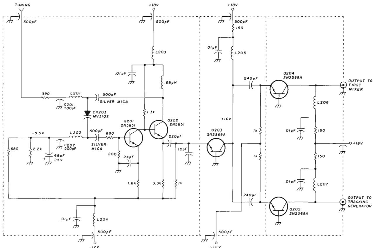
fig. 9. VCO schematic. Range is 200-300 MHz. CR203 is a Motorola MV3102. C201 and C202 are 500-pF feedthrough bypass capacitors. L201, L202: 1 turn no. 18 AWG (1mm) wire. L203-L207: 5/2-turn chokes.
