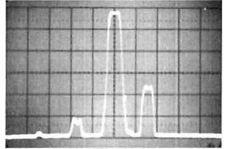
fig. 26. Output of a commercially made 55b transmitter into a 50-ohm load with carrier inserted at about 3.8 MHz. Scan 500 kHz/division. Note spurious signals at about 3050 kHz and 4550 kHz.
