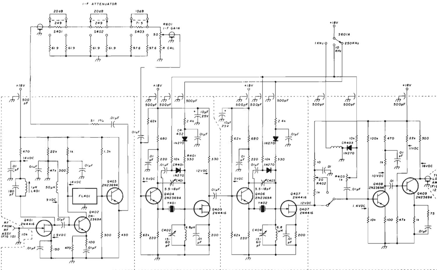
fig. 11. I-f section schematic. All resistors in the attenuator must be 1% tolerance. Resistors must be added in series or parallel to obtain 51 ohms  $\pm 1\%$  with R601. Feedthrough caps are 500 pF.
