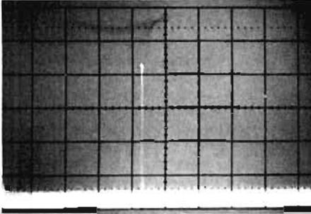
fig. 21. Setup is as shown in fig. 27. I-f gain has been reduced to take advantage of the full dynamic range.
