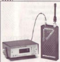
*Measuring DTMF Tone with decoding unit*
