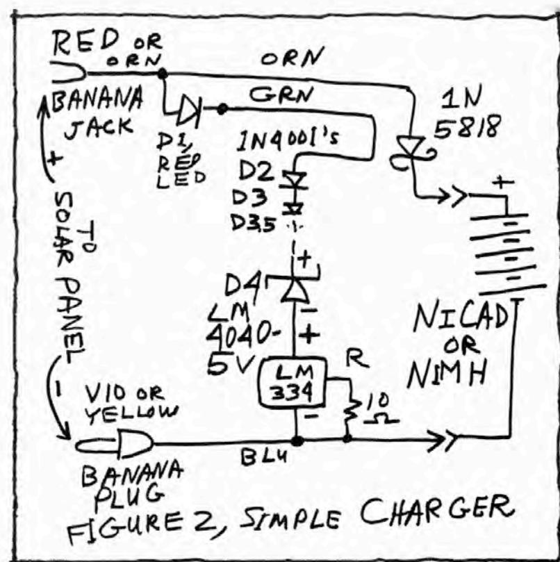
and holding the voltage low. But if the voltage is above 10 V, the LED will turn on, indicating that the battery is NOT getting charged. This is a bad thing, so the LED signifies bad news. It's time to re-adjust the rubber bands! I mount the LED right near the banana plugs, which I keep outside of my pack's back pocket, while the battery rides inside the pocket. The solar panel is lashed on top of my pack.
