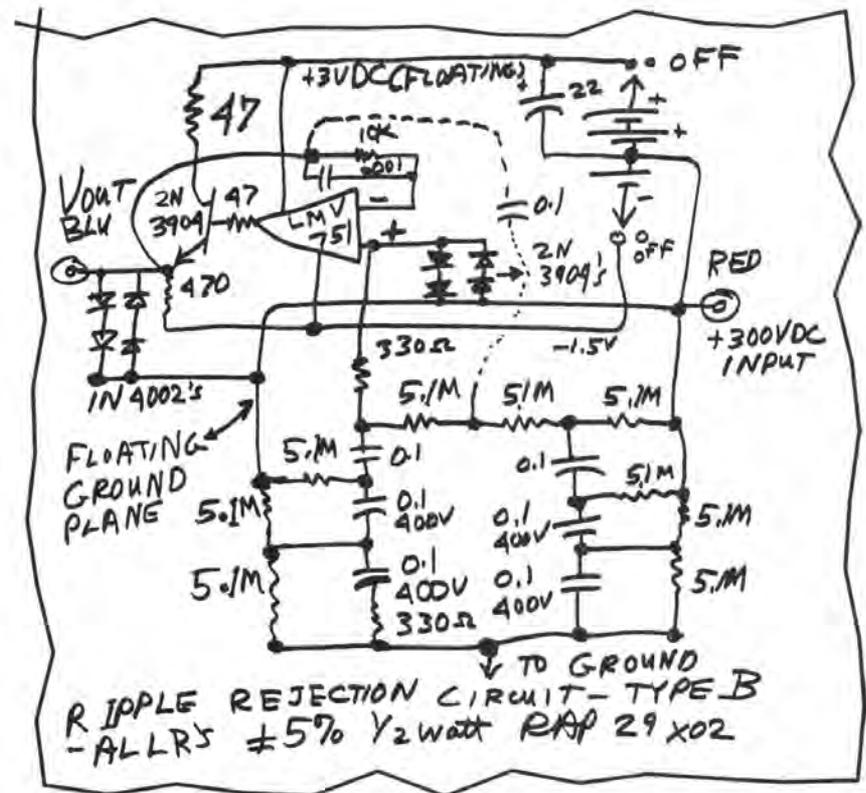
ripple-rejection, using my NoiseMaker (schematic is on my Web site) to try to cut the ripple of an 85-mV p-p (26-mV rms) noise at a 26-kHz nominal switching frequency, with lots of harmonics at 52 and 78 kHz. Although the Type A circuit improved the 26 mV to 0.88 mV, Type B did a bit better at 0.83 mV. But that was NOT unexpected. So it's not too hard to get a 30-dB noise improvement by employing a cheap, low-noise op amp, such as LMV751.
