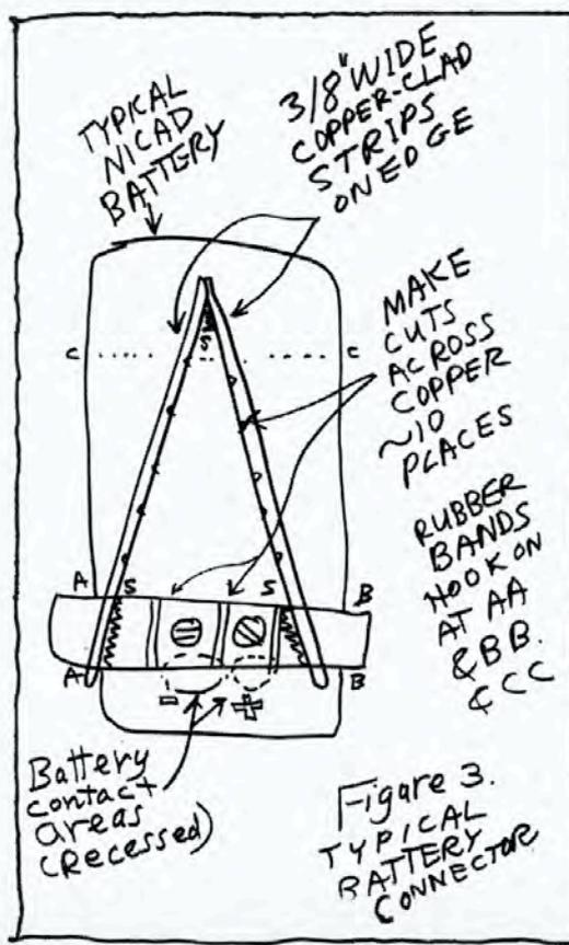
I used tin snips to cut copper-clad 1/16-in. epoxy material into thin strips, such as 3/8-in. wide. And I used a hack-saw blade to saw a dozen gaps in the copper. I soldered three of these thin strips (at the places marked with
