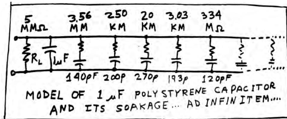
age is a big capacitor, in parallel with several small capacitors in series with various large resistors (see the figure). If we put a dc voltage on the capacitor for 0.1 second, some of those smaller capacitors will be charged up, but some of the bigger ones will take more time.
