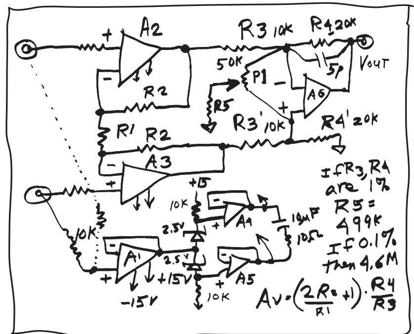
A2 and A3. So, your "preferred embodiment" could put in a couple LMH6624s and get very low voltage noise, such as 1.4 nV/Hz, total for the whole circuit, assuming your  $R_S$  is lower than 200 .
