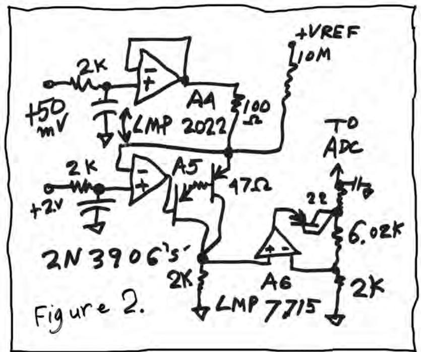
resistors, the common-mode rejection ratio (CMRR) of the third amplifier can be as poor as 37 dB with respect to the input or 31 dB at the output. They said they were assuming there would not be much CM noise.
