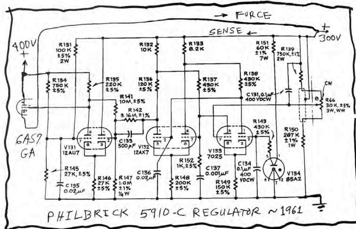
high-line. Also, it has submillivolt gain error, for line, load, or ripple.
