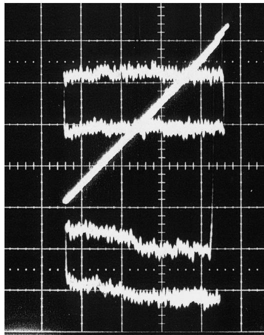
3. LMC6042,  $F = 0.6$  Hz; output  $\pm 4$  V into  $1\text{ k}\Omega$  (lower trace); upper trace,  $2\text{ }\mu\text{V p-p}$  at  $20\text{ }\mu\text{V/div.}$ ; lower trace,  $6\text{ }\mu\text{V p-p}$  at  $20\text{ }\mu\text{V/div.}$
