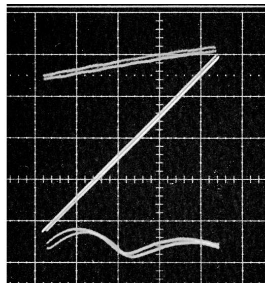
our first CMOS amplifiers (*Fig. 2*). Like the LM301A, its gain degrades when overloaded with 1 k $\Omega$ . But the nonlinearity (deviation from best straight line) is only 18  $\mu$ V p-p. That's not bad for an 8-V, 8-mA p-p swing.
