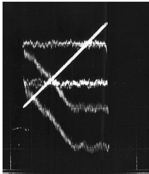
an LM301 can make a unity-gain inverter with a nonlinearity of 1.2 ppm. At lighter loads, it's even better.
