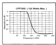
The input signal for the model LPF7002 should not exceed 125 watts. Use on higher powers can permanently damage the filter and will void the warranty.
