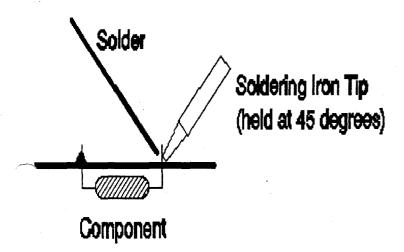
to the tip of the cone as possible. **Important.** In R.F. construction, solder components as close to the board as possible, <u>unless otherwise instructed</u>, or the circuit will be prone to instability due to extra lead length adding spurious inductance and capacitance.
