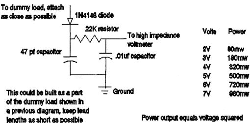
Power output equals voltage squared dvided by 50 (presuming you have a 50-52 ohm dummy load) source material is. If you do nothear anything, check your connections. We have found that the 1/8 point is best for most audio sources and will help prevent over modulating (a limiter is needed to fully prevent this) the transmitter.
