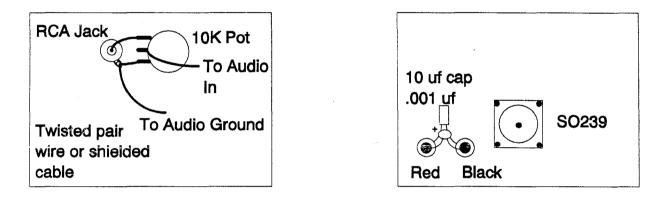
Follow the wiring diagram for the audio input. Two leads will go to the PLL board, audio in and ground. These can be either twisted pair or shielded 2 conductor cable.
