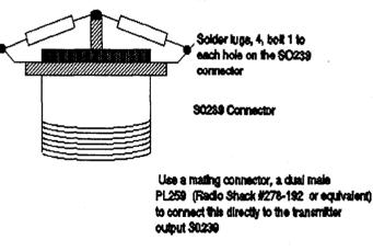
\*If 2 watt resistors are used, this load can be used with transmitters with an ouput power of 5-6 welfa maximum.
